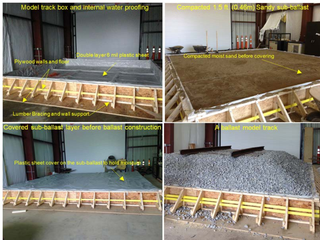
Figure 5. Photos Showing the Construction of a Ballast Model with the Lined Box for the Sub-Ballast (top left), Filled Sub-Ballast Box (Top Right), Filled and Lined Sub-Ballast (Bottom Left), and Complete Model (Bottom Right)
