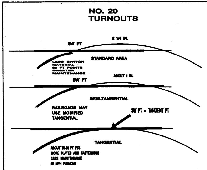
Figure 4 The tangential concept
