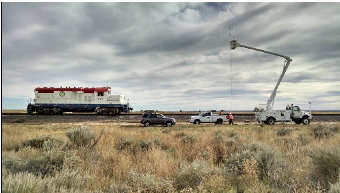
Figure 13. Field Testing with an ACSES Radio on the Locomotive Desensing an ITC Wayside Radio
