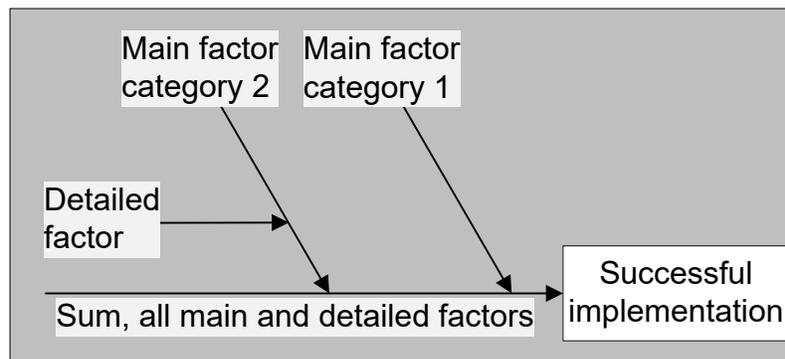
**Figure 15. Structure of an Ishikawa Diagram**
