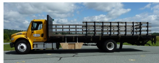
Figure 6. Flatbed truck with hang-up feature attached
