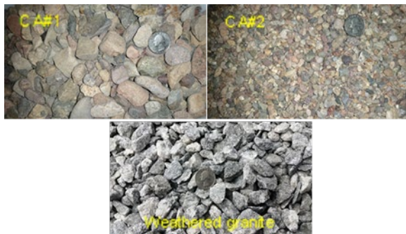
Figure 1. Aggregates: CA#1 and CA#2 (Tucson, AZ); weathered granite (size 57/67, Anderson, SC)
