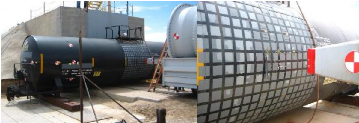
Figure 8. Overall Test Setup (left) and Ram Arm with 12- by 12-inch Indenter Aligned with Center of the Tank Car (right)
