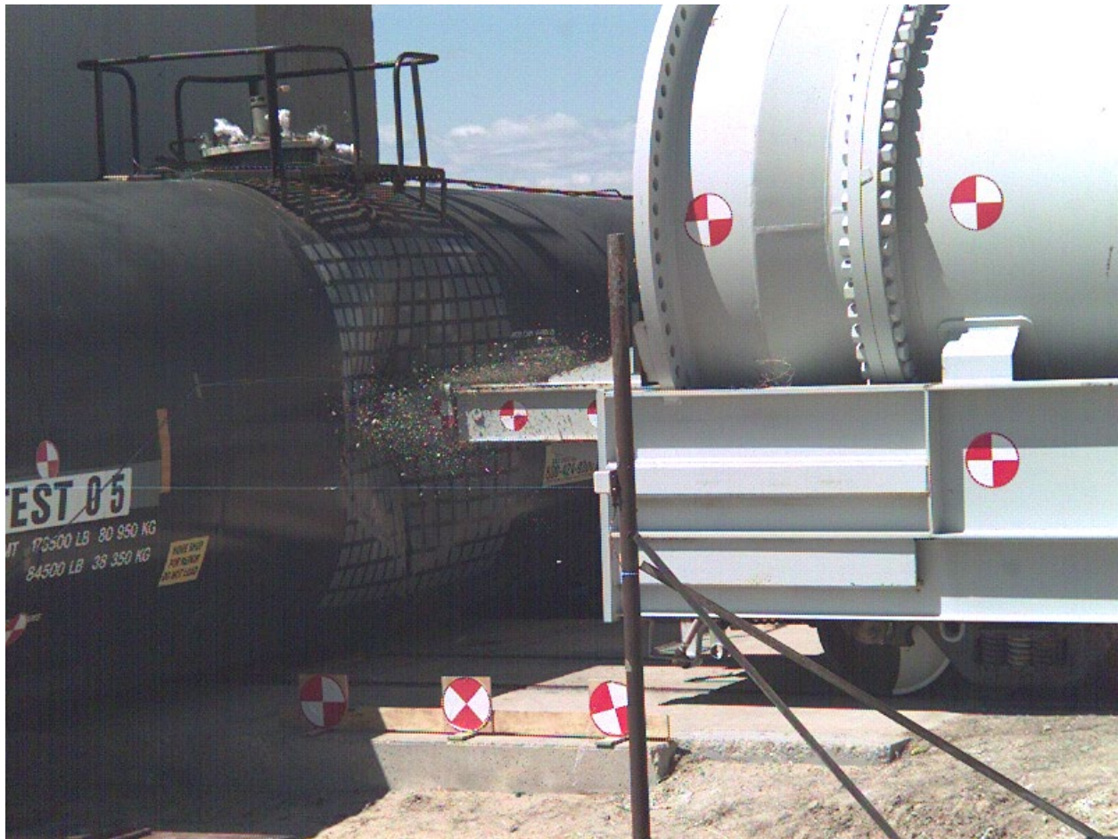
Figure 14. Deformed Tank Just Prior to Puncture
