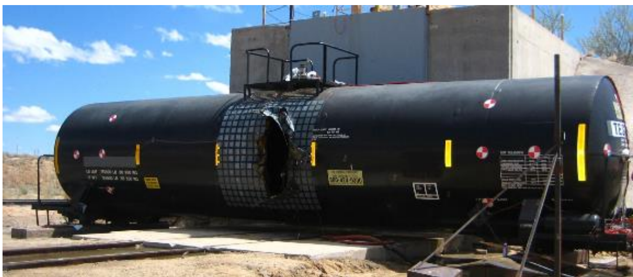
Figure 15. Tank Car—Post Impact (impact side)
