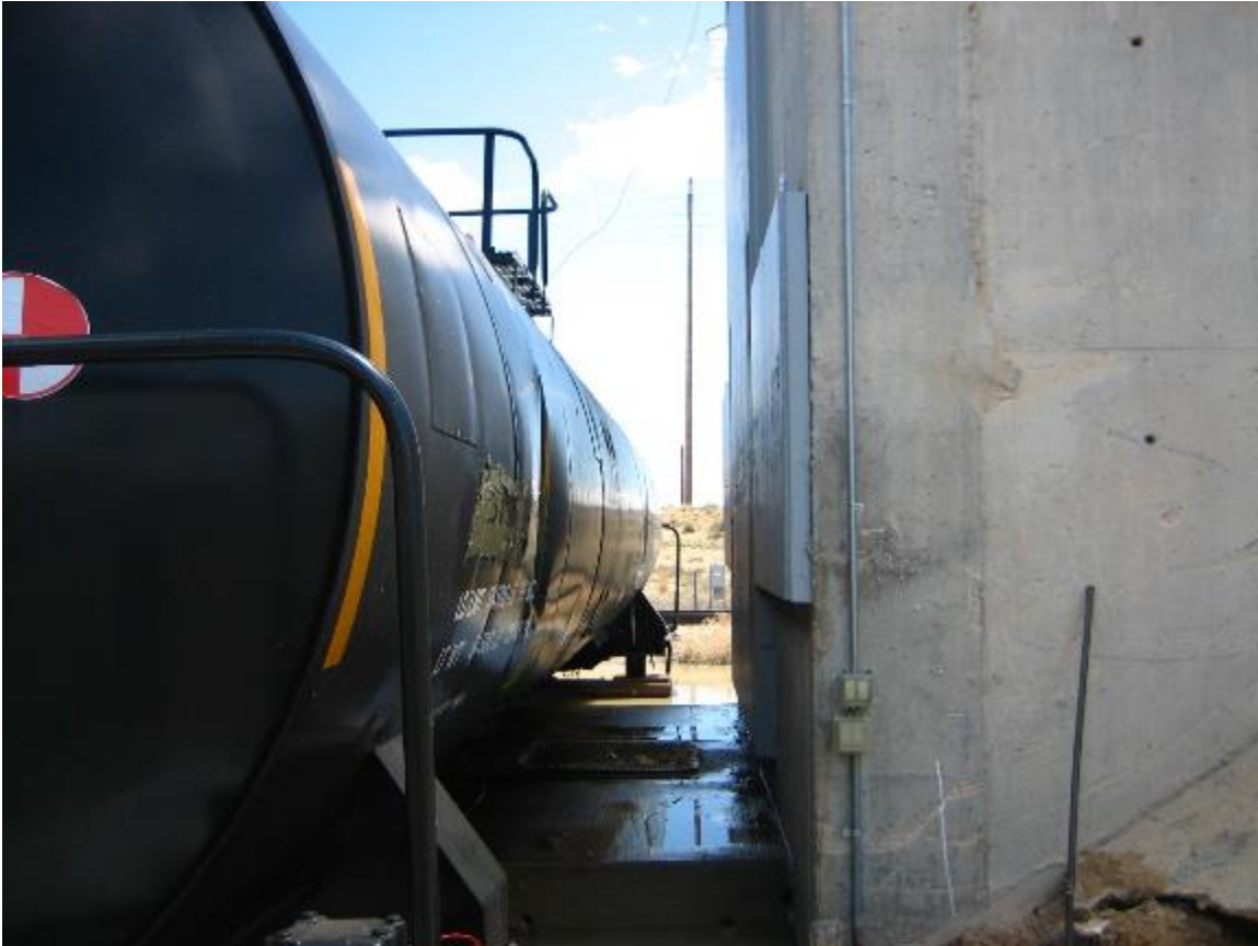
Figure 16. Tank Car—Post Impact (wall side)
