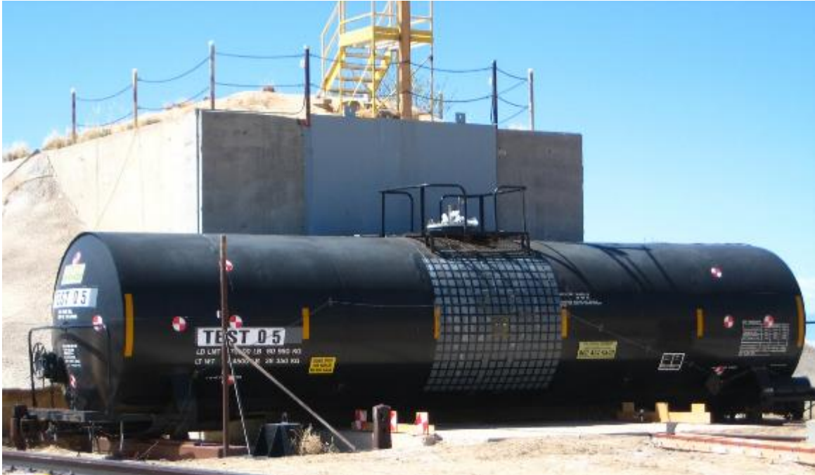
Figure 4. Target Tank Mounted on Support Skids
