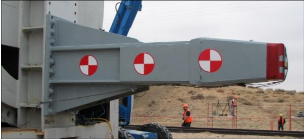
Figure 7. Ram Arm with 12- by 12-inch Indenter (from previous test)
