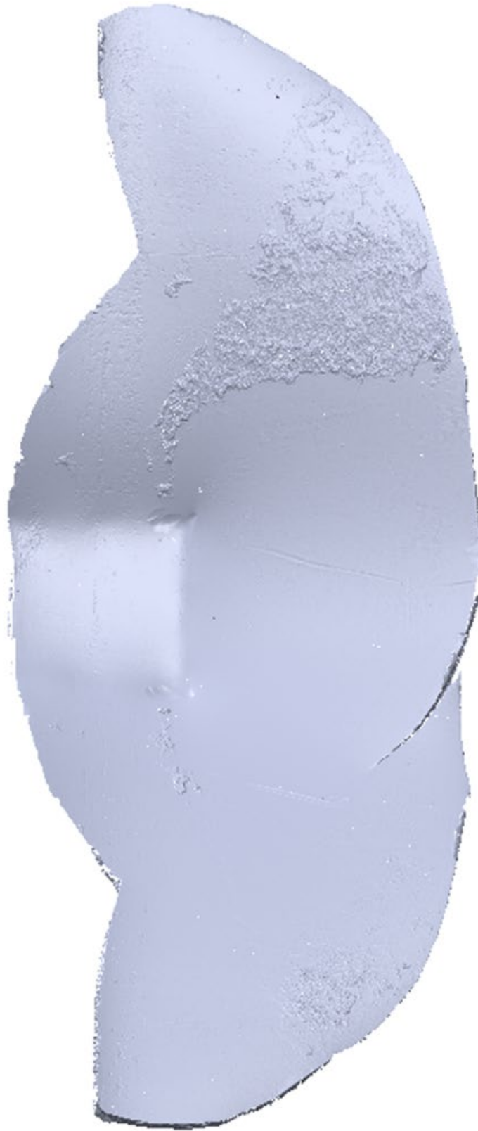
Figure 31. Scanned Geometry of Ejected Panel Segment
