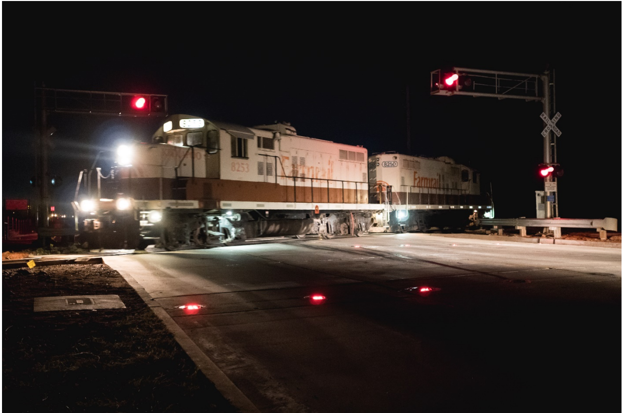
Figure 3 – Elk City in-pavement lights, looking west
