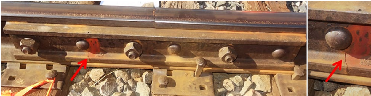
Figure 6. Bolt Hole Defect on a Standard Design Bar
