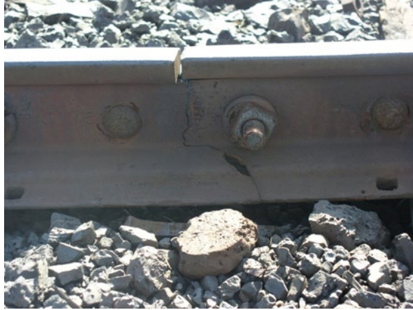
Figure F-6. Illustration of Long Toe Angle Joint Bar with Center Crack
