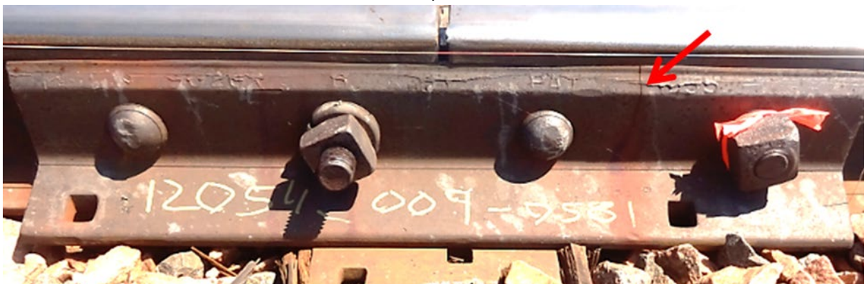
Figure 5. Quarter Crack on a Long Toe (Angle) Bar Originating at the Top of the Bar
