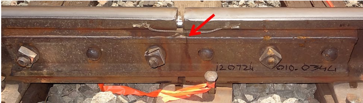
Figure 2. Top Center Defect on a Standard Design Head-Free Bar
