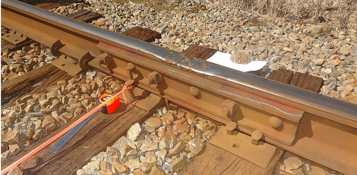
Figure 9. Large Rail End Batter at a Failed Rail Joint Location
