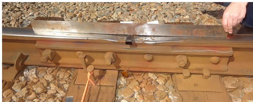
b) Rail End Batter Magnitude Illustration
