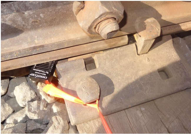
b) Measurement of Gap between Rail Base and Tie Plate
