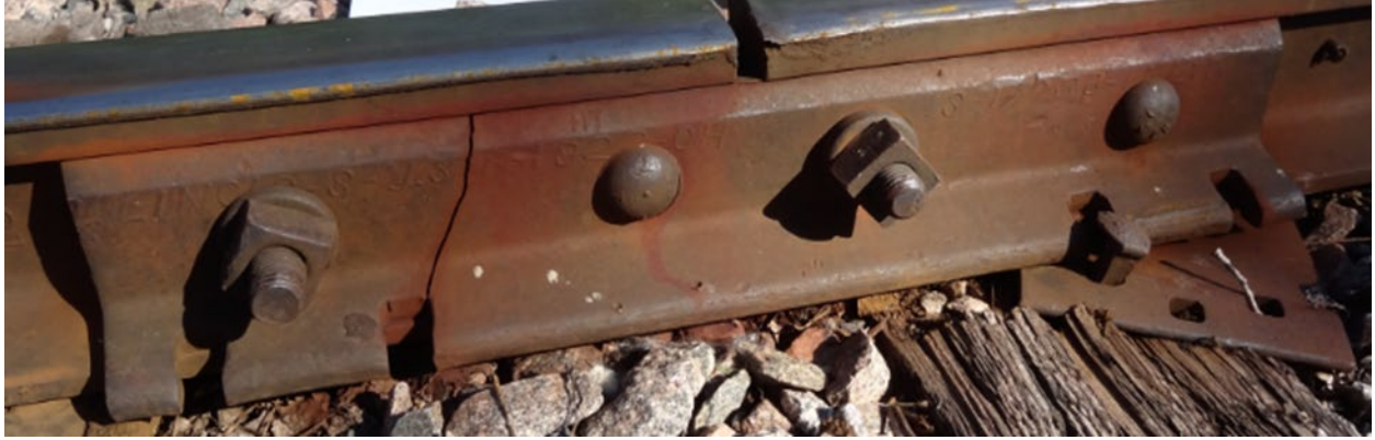
Figure 3. Full Quarter Break on a Long Toe (Angle) Bar
