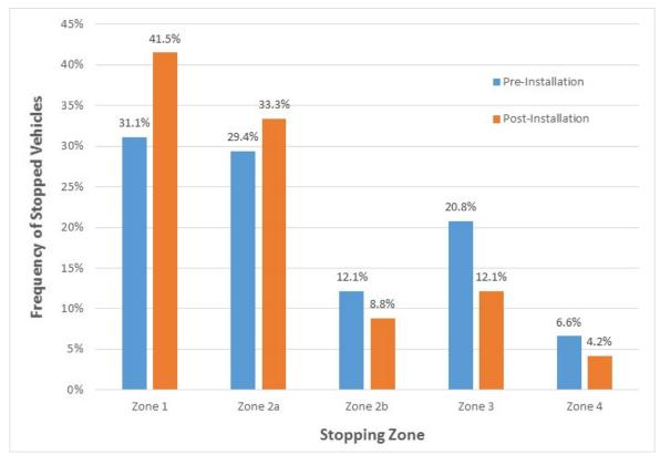
Figure 12. Frequency of Southbound Vehicles Stopping by Zone
