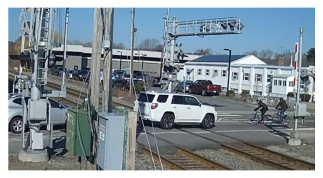
Figure 13. Example of Northbound Vehicles Stopping on Tracks Due to Bicyclists
