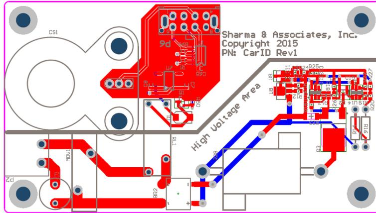
Figure 7-13 – Car ID Module PCB Design Layout
