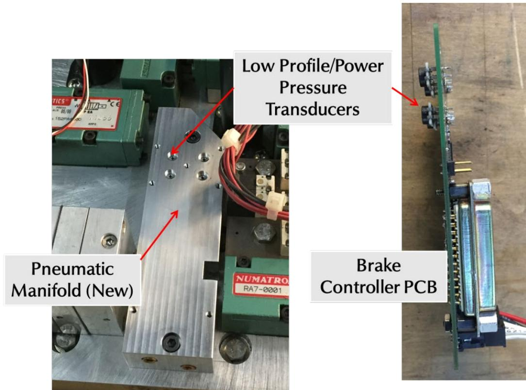
Figure 7-3 – Brake Controller Manifold and Pressure Transducers
