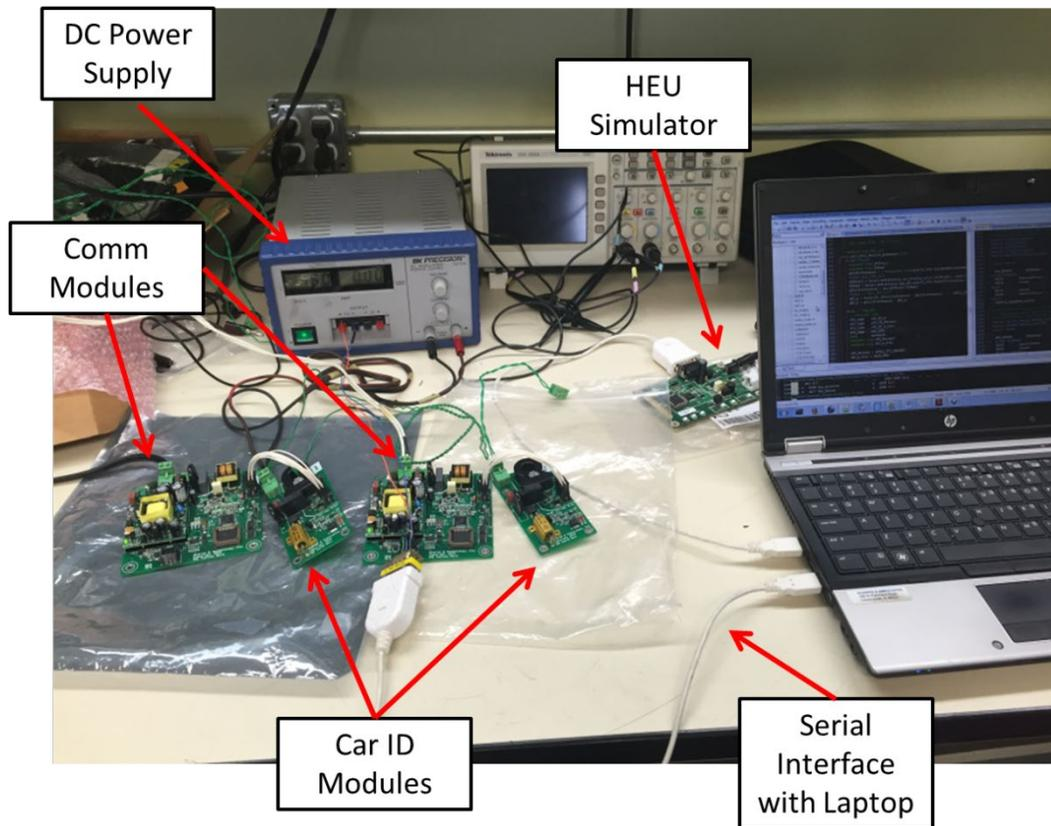
**Figure 8-1 – Representation of Software and Hardware Testing**
