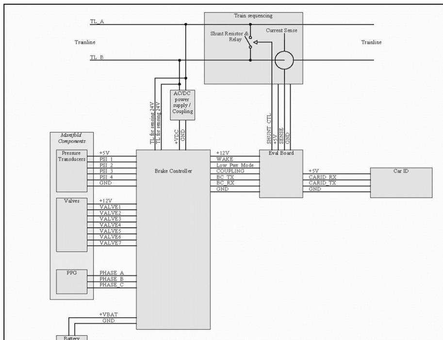
**Figure 5-1 – Proposed CCD Architecture**
