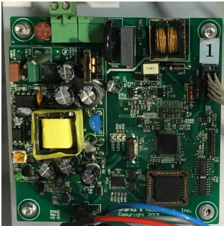
**Figure 7-9 – Comm Module Board**
