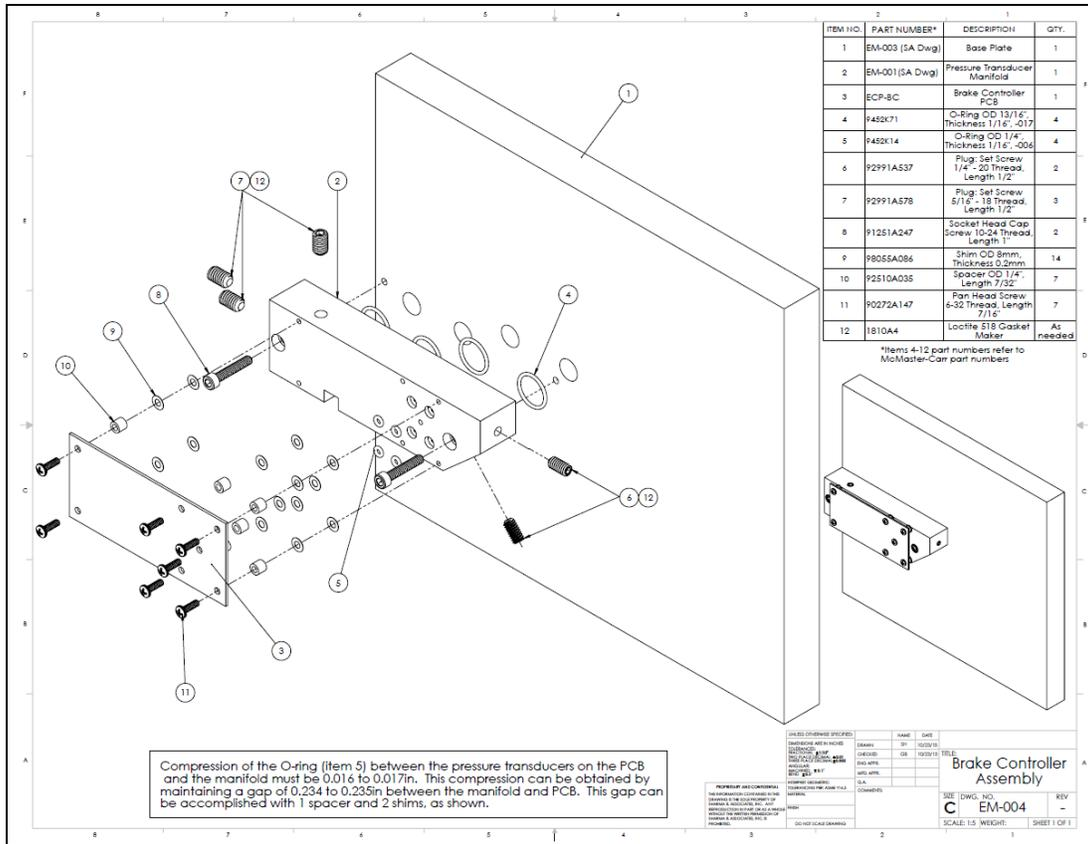
**Figure 7-4 – Brake Controller Assembly with Manifold**
