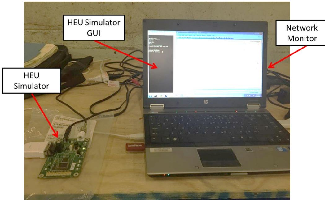
**Figure 9-3 – ECP Testing with the HEU Simulator**
