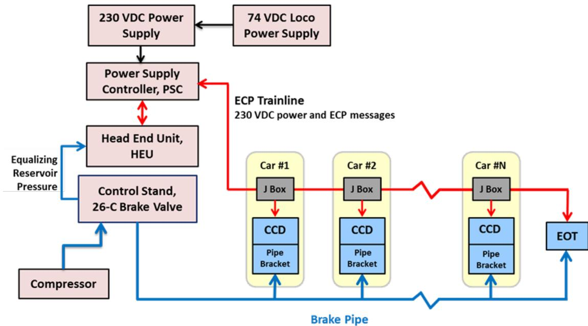
**Figure 2-1 – Generic ECP Train System Layout**
