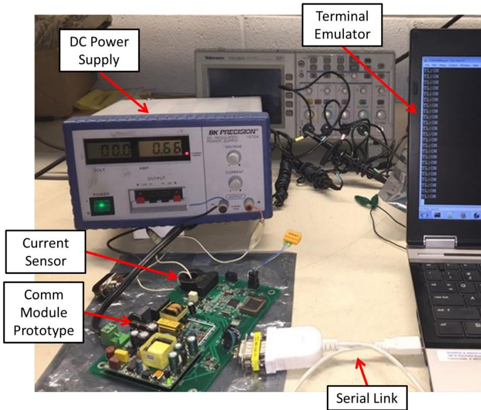
**Figure 8-4 – Preliminary Current Sensor Testing for Car Sequencing**
