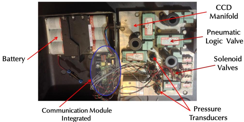
**Figure 4-2 – Emulator CCD, as Received**
