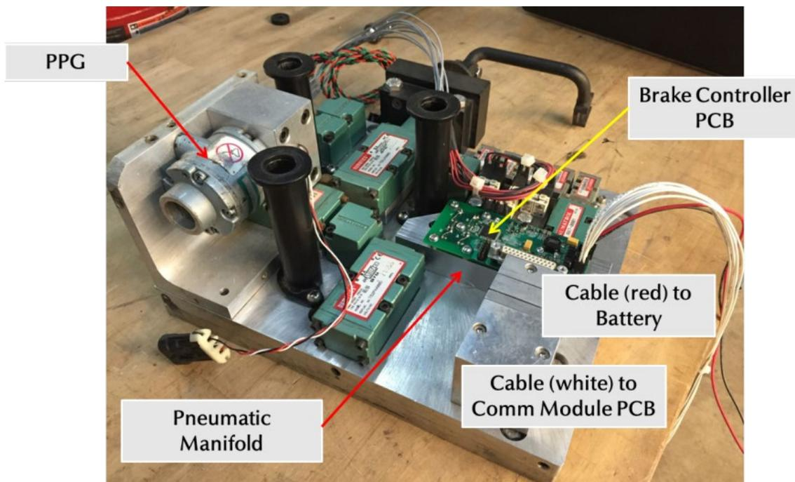
**Figure 7-6 – CCD with Brake Controller and PPG Mounted**
