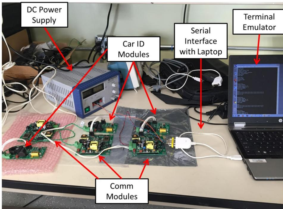
Figure 9-5 – Testing Car ID Read and Write Operations
