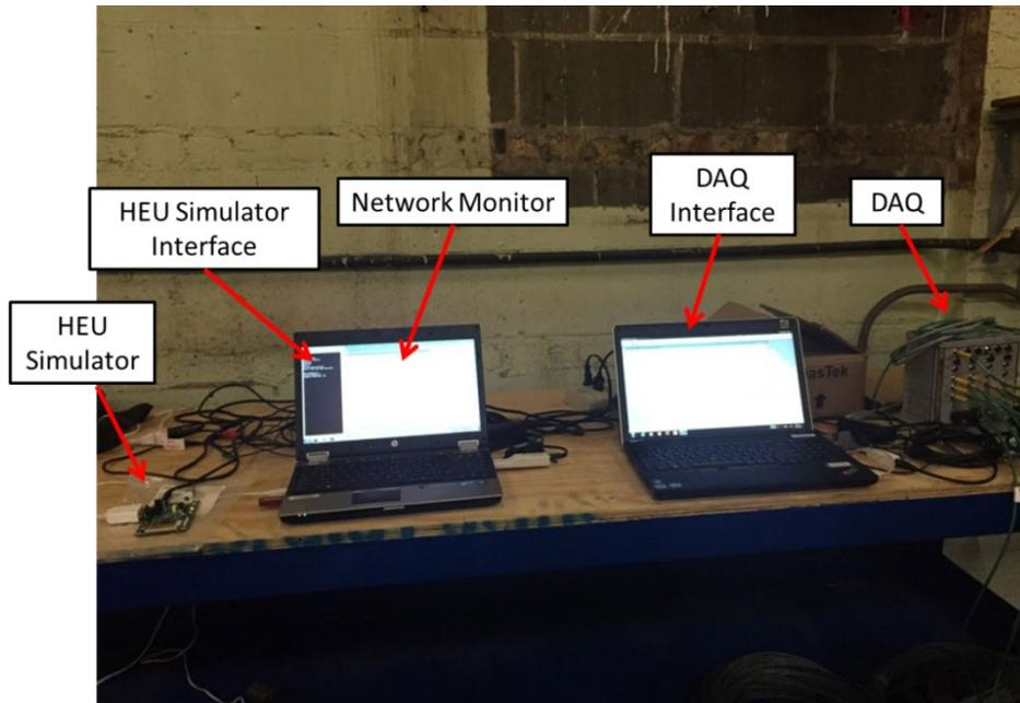
**Figure 9-8 – ECP System Testing Using a DAQ**
