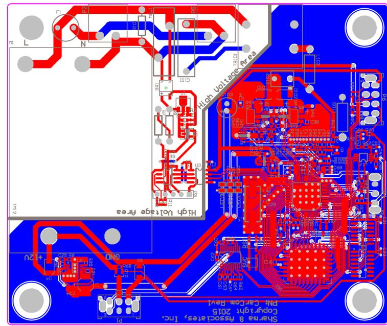
**Figure 7-7 – Comm Module PCB Design Layout**
