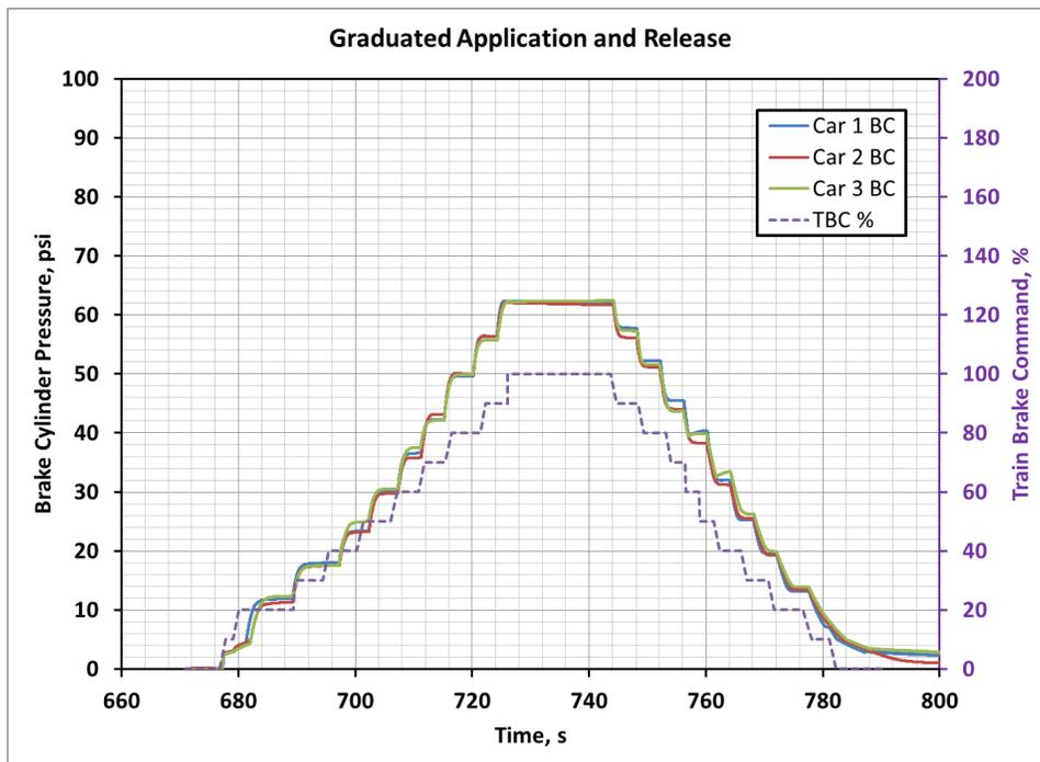
Figure 9-10 – Graduated Full Service Brake Application and Release
