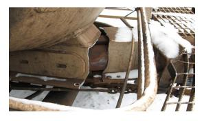
Figure 1. Example of a cracked sill
