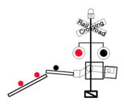
Track Speed; Gate arm tip broken outside of flashing gate lights.
