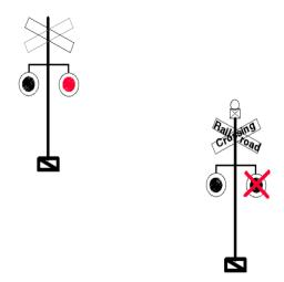
Partial Activation, single pair of flashing lights on approach to crossing, no back lights visible.
