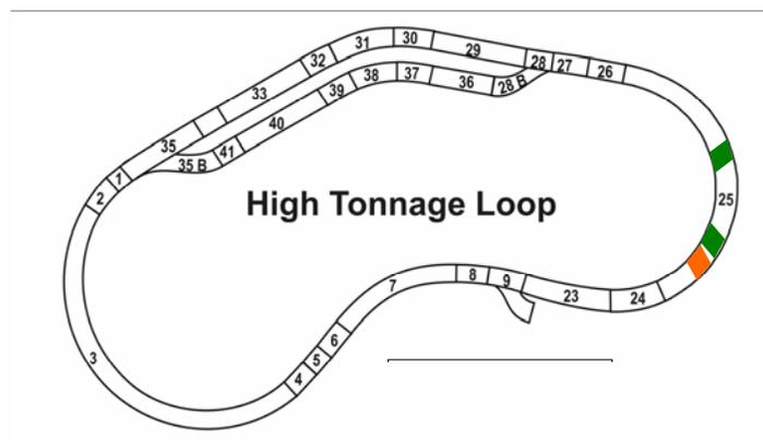
Figure 1. Test Tie Locations on HTL.
