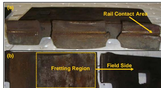
Figure 2. Rail Contact and Tie Plate Fretting Regions
