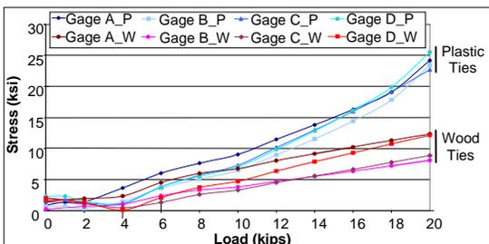
Figure 6. Maximum Principal Stress for Half-Tie Test.
