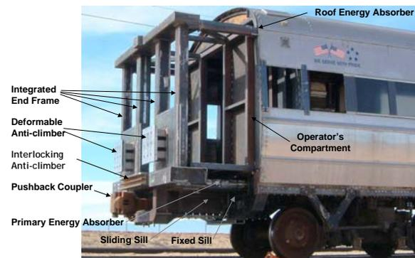
Figure 2. Cab Car Crush Zone
