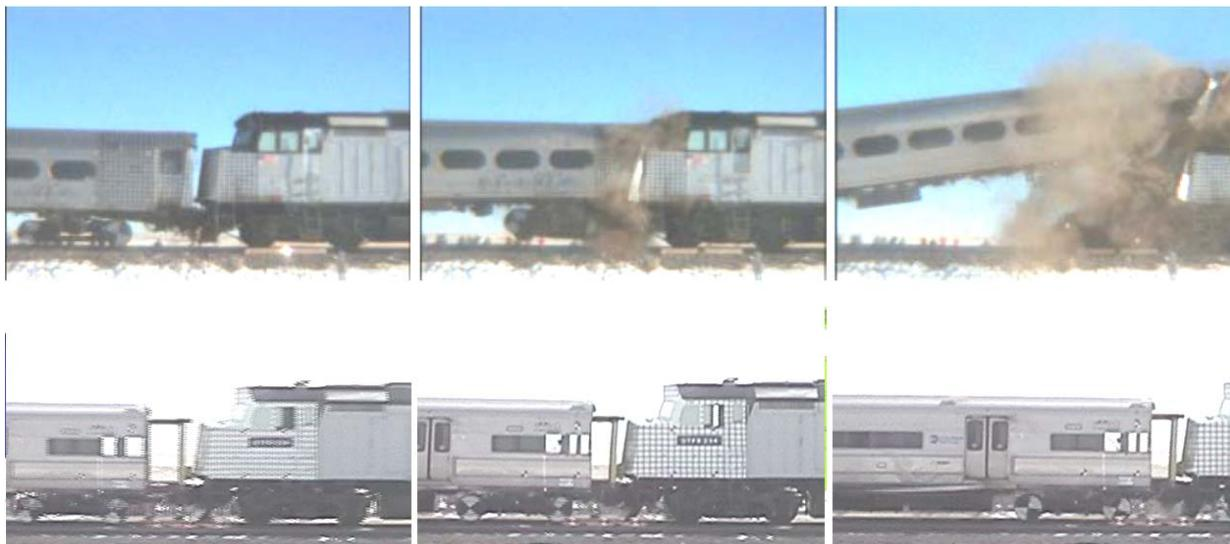
Figure 1. Frames from Train-to-Train Test Movies of Conventional and CEM Equipment
