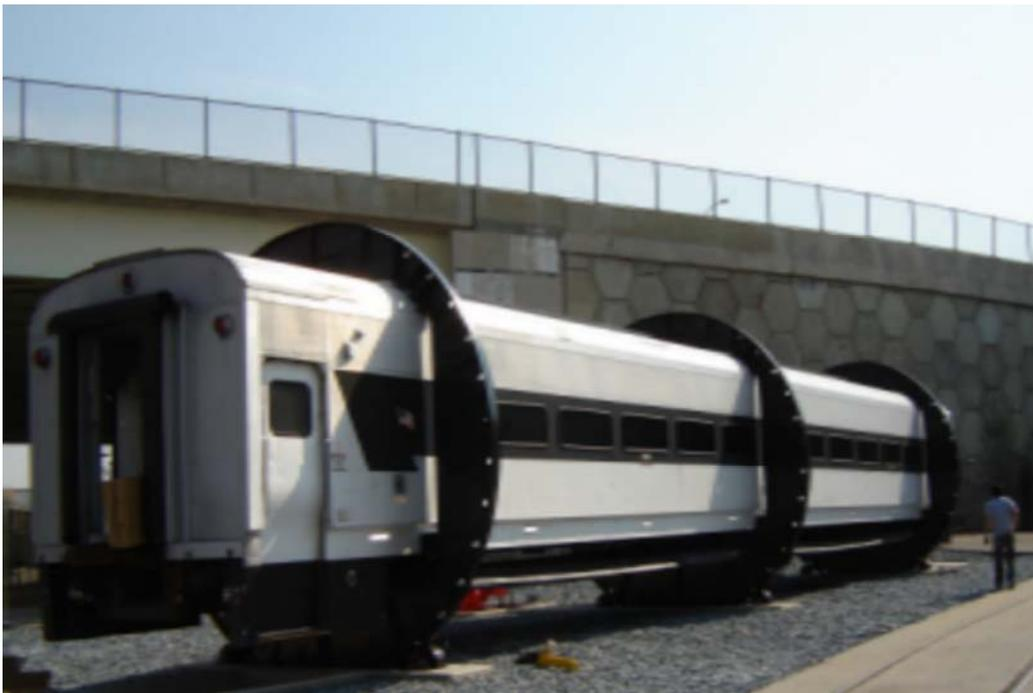
*Figure 1. Emergency Evacuation Simulator (Rollover Rig), WMATA, Landover, MD*
