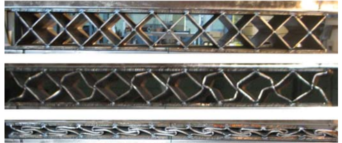
Figure 6. Progressive Crush on Diamond Core Sample
