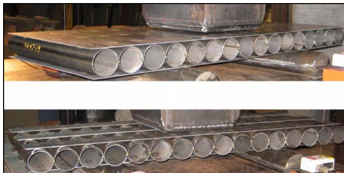
Figure 13. Pipe Core Sandwich Panel with Solid (top photo) and Strip (bottom photo) Facesheets
