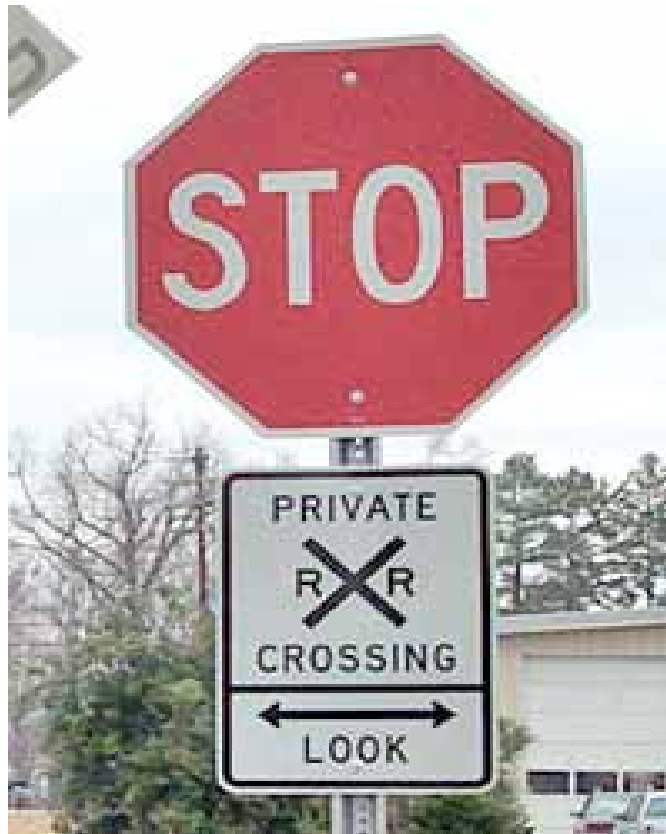
Figure 4. Private Grade Crossing Stop and Cross Buck Sign Treatment (15)
