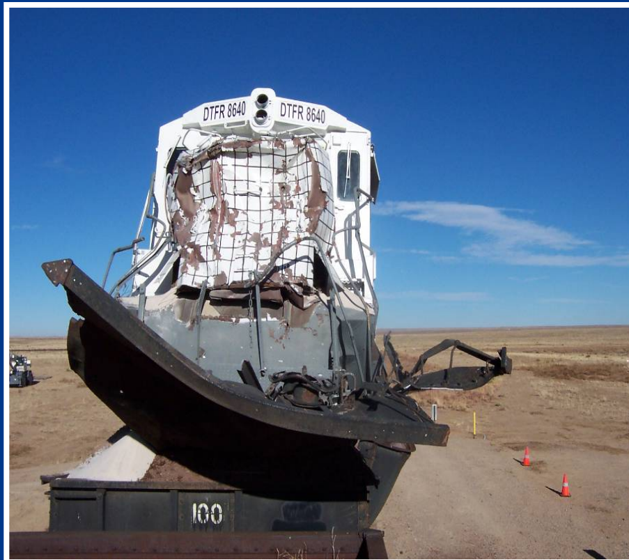
Extensive damage to the front end of the locomotive
