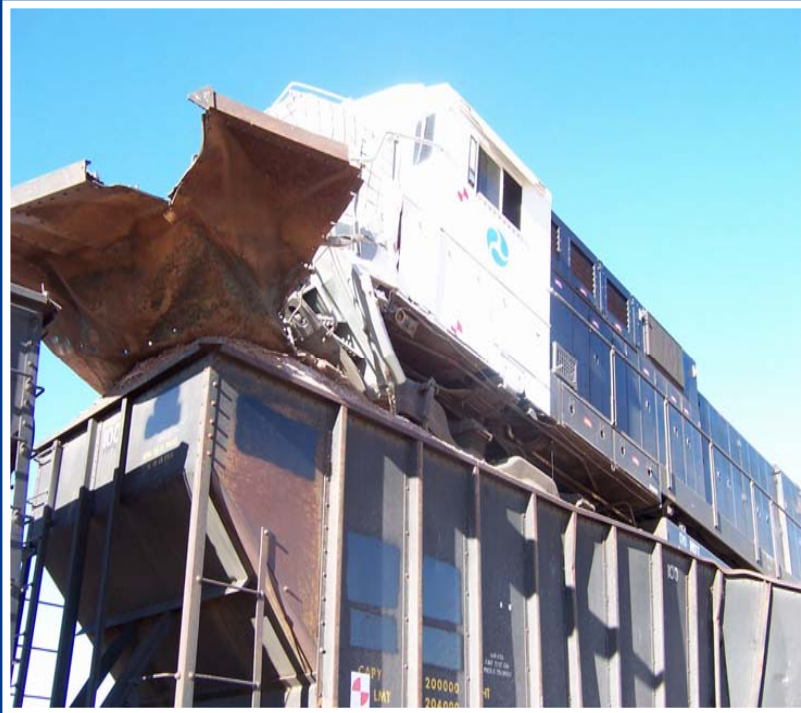
Position of locomotive following collision test
