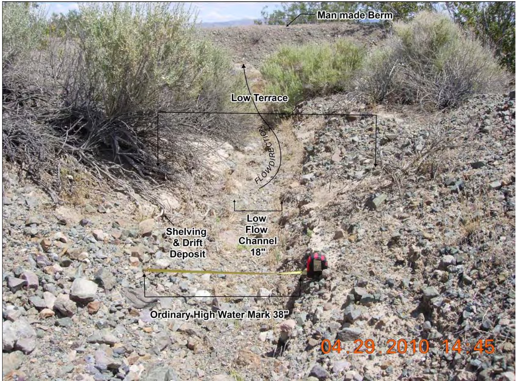
Exhibit A. Figure 8. Typical examples of field indicators of active surface water flow and Ordinary High Water Marks found within ephemerals drainages occurring within the DesertXpress Project Study Area.
