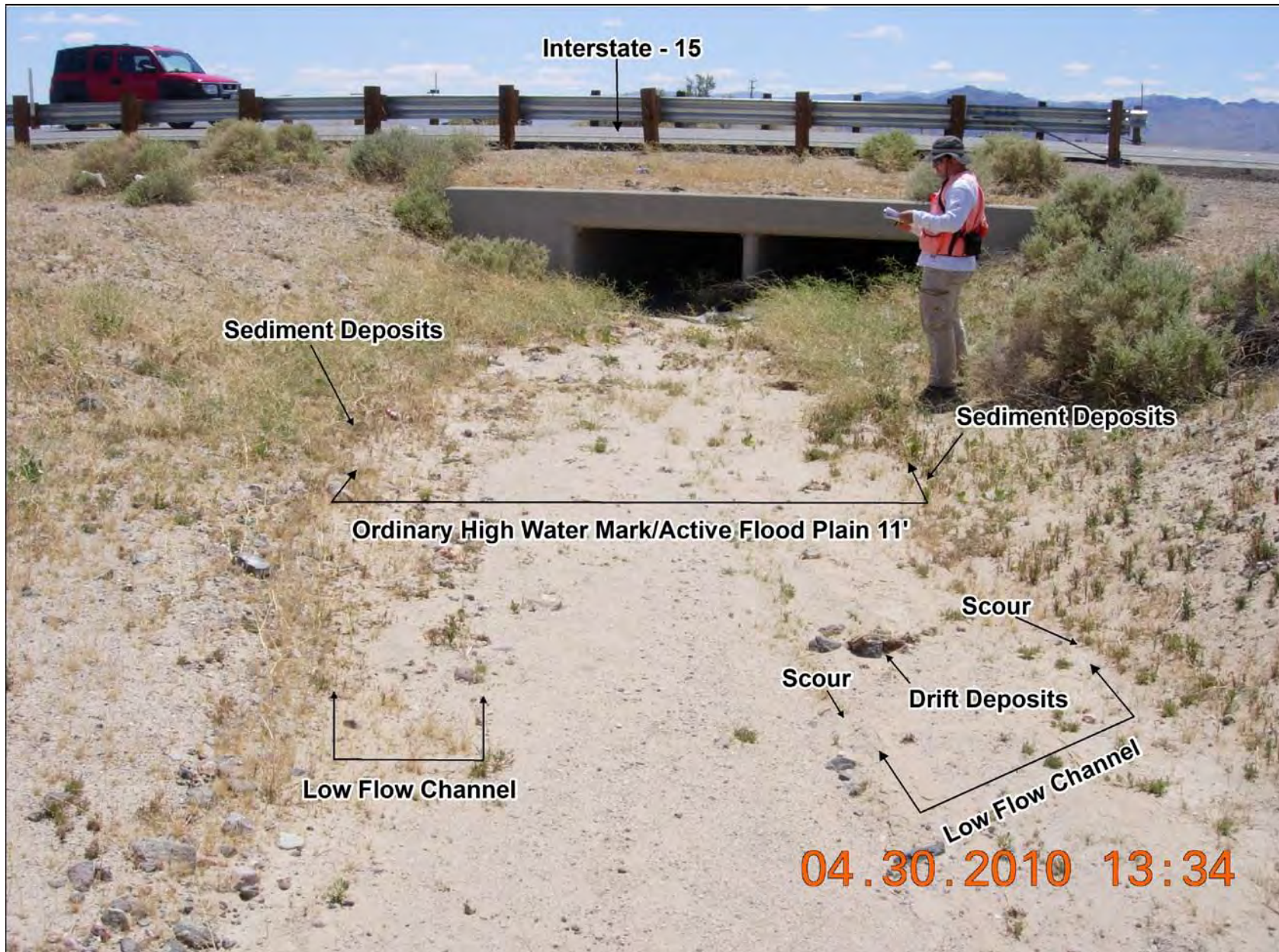
Exhibit A. Figure 12. Typical examples of field indicators of active surface water flow and Ordinary High Water Marks found within ephemerals drainages occurring within the DesertXpress Project Study Area.
