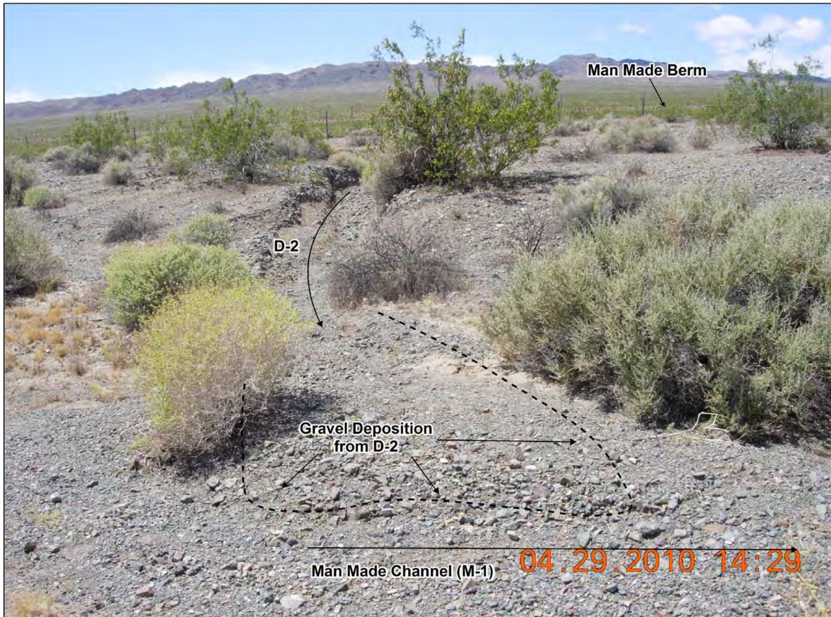
Exhibit A. Figure 6. Typical examples of field indicators of active surface water flow and Ordinary High Water Marks found within ephemerals drainages occurring within the DesertXpress Project Study Area.
