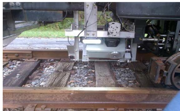
Figure 4. NCRTM Sensor Mounted Under R-4
