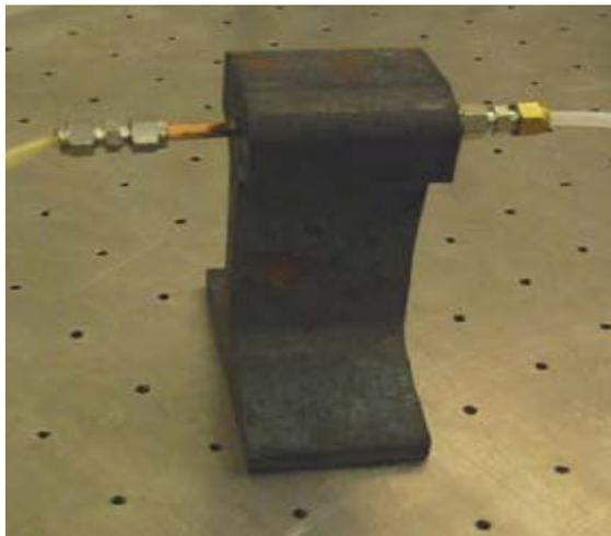
Figure 2. Instrumented Short Rail Section for Lab Test
