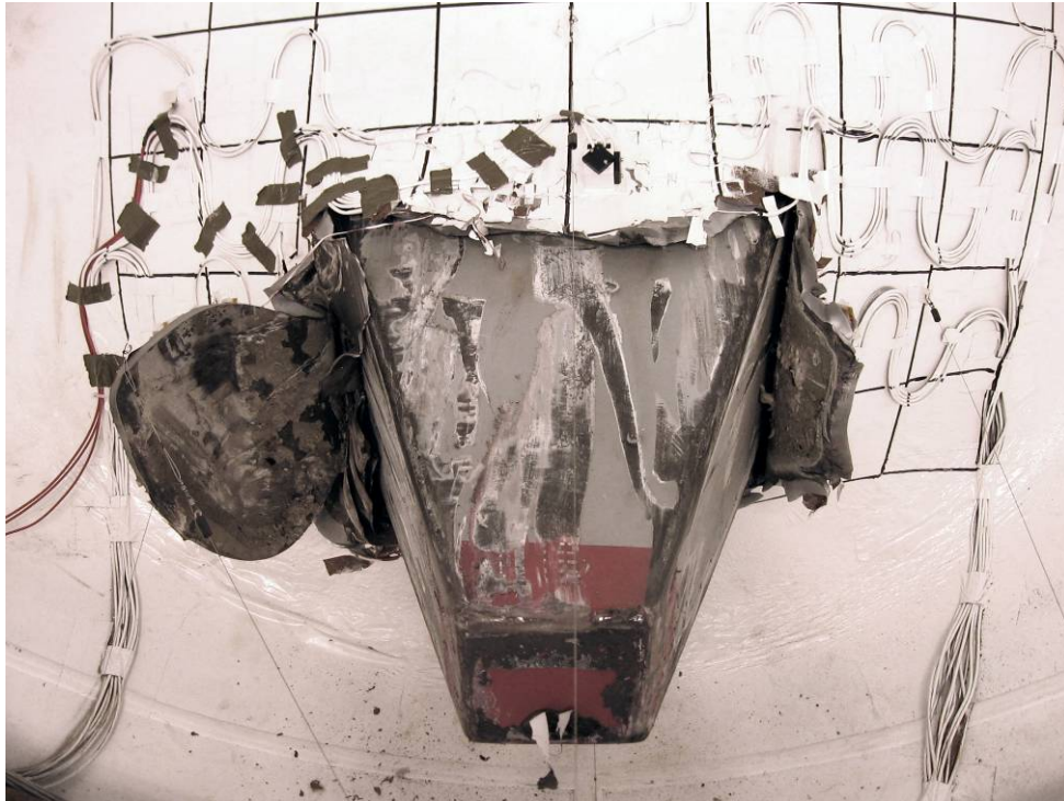
Figure 273. Internal puncture of the tank head in Head Test 3.
