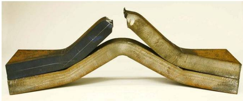
Figure 91. Observed BFCM specimen deformations at different impact velocities.
