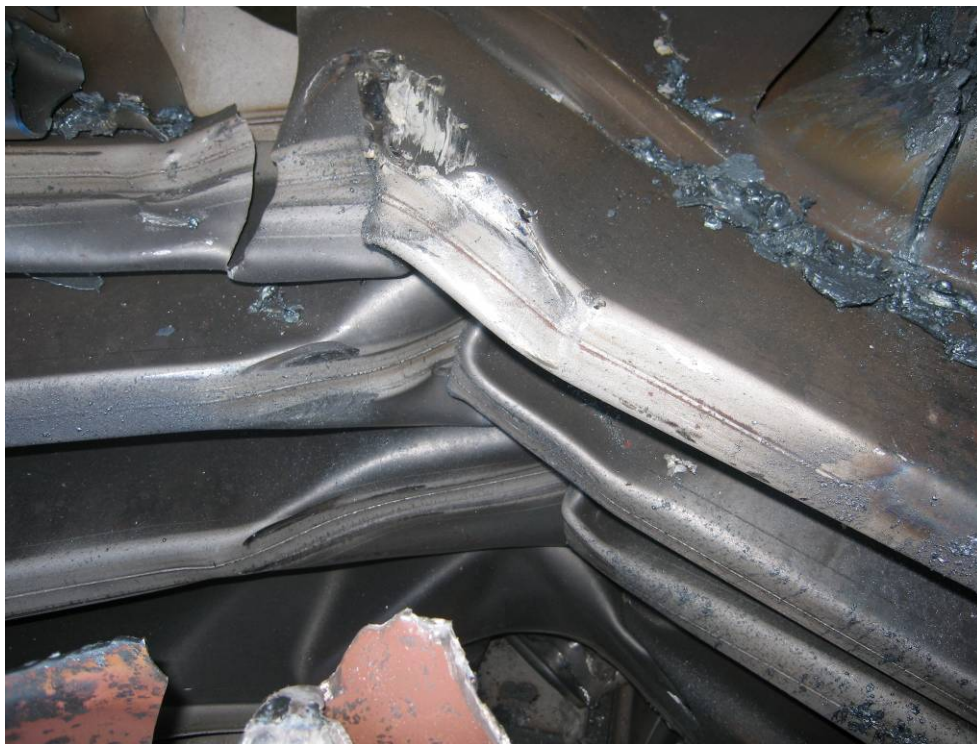
Figure 276. Buckling of the end EMS corrugation in Head Test 3.
