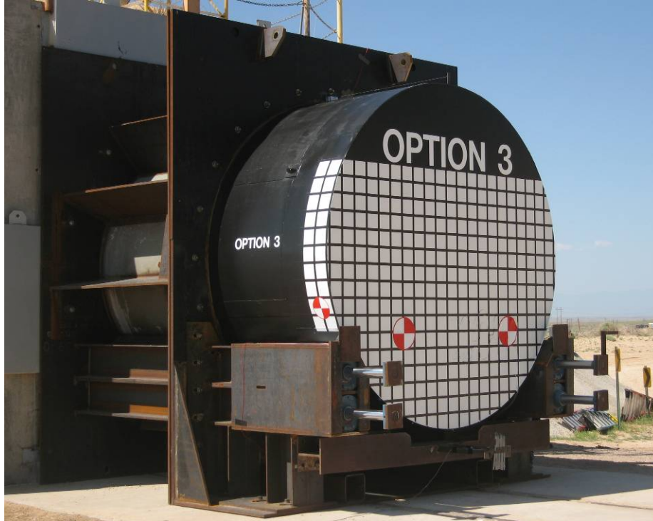
Figure 270. Pretest configuration of the test head and corrugated EMS system.
