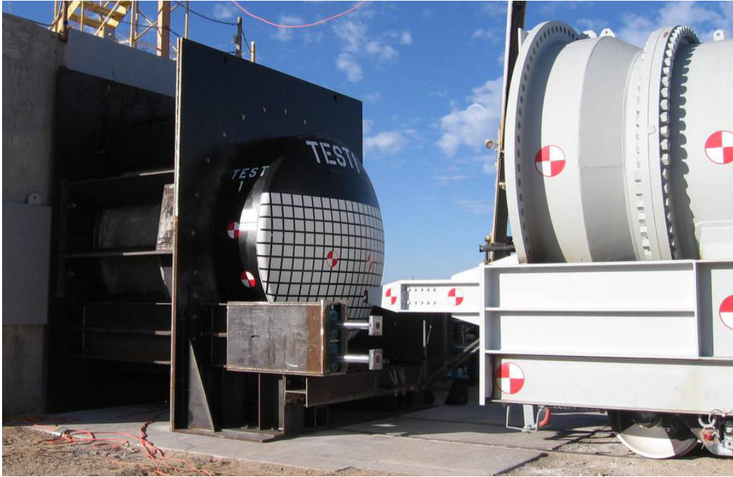
Figure 148. Pretest conditions of the test article and ram car for Head Test 1.
