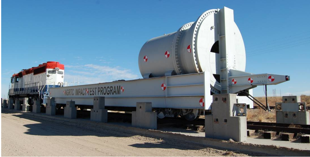
Figure 46. Modified ram car and ram head used in Test 2
