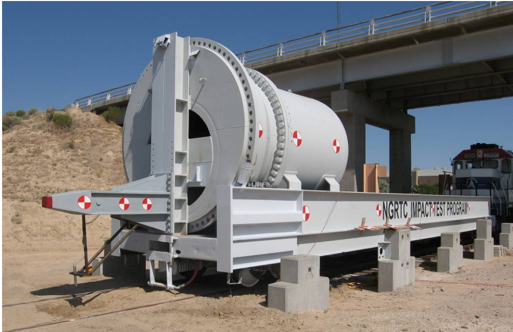
Figure 271. Pretest configuration of the test head and corrugated EMS system.
