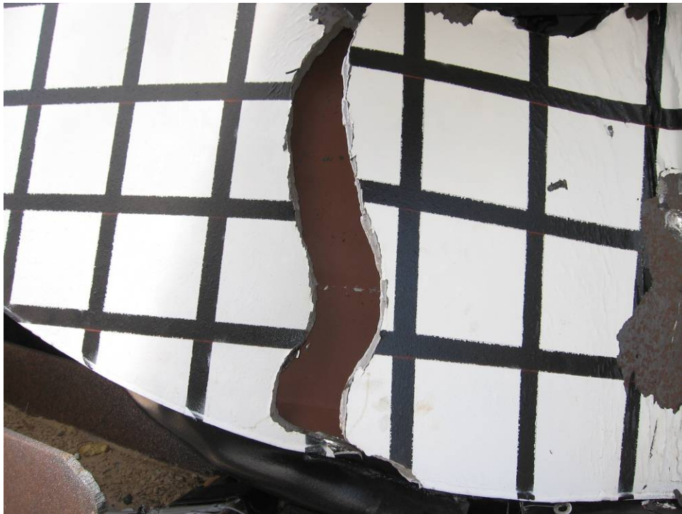
Figure 277. Fractured EMS end cover plate in Head Test 3.
