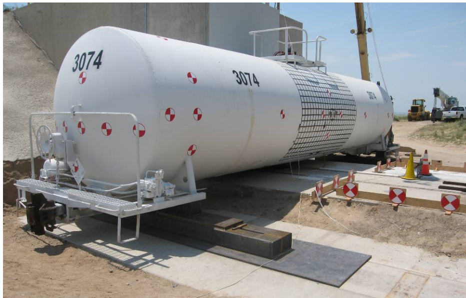
Figure 45. Test 2 target Tank Car 3074 mounted on support skids.
