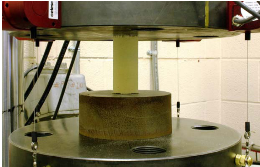
Figure 193. Dual platen setup for unconfined compression testing of foam [70].
