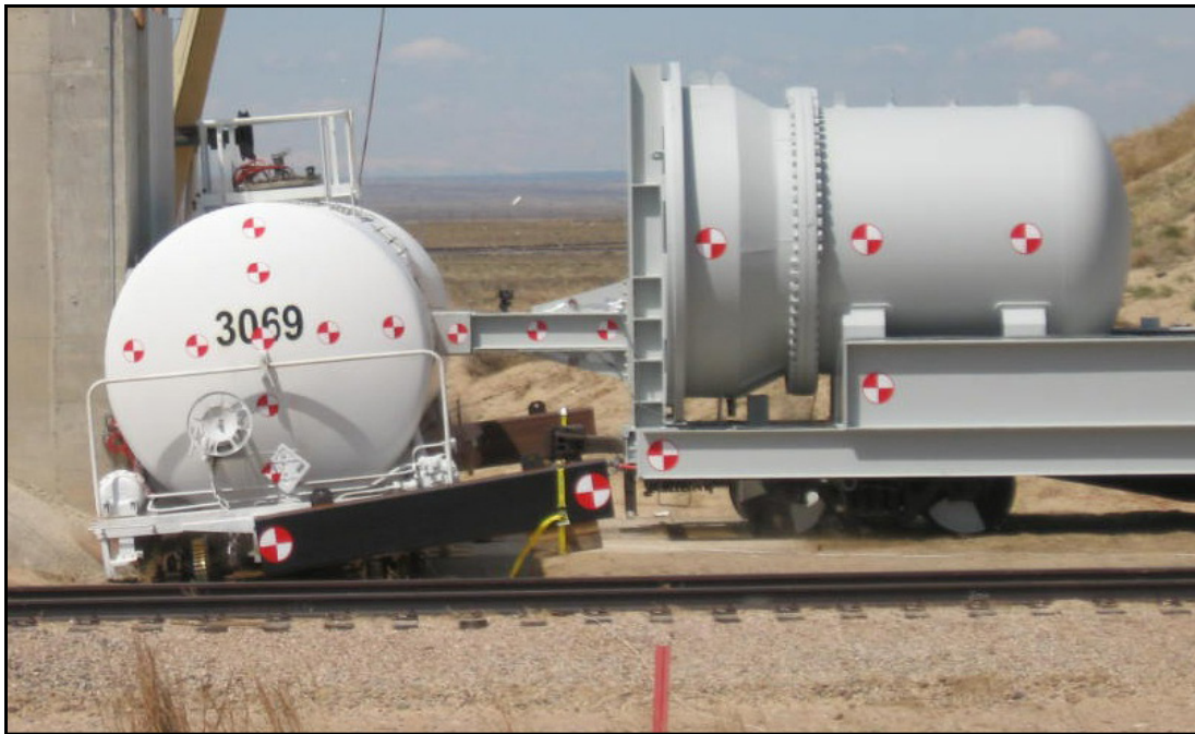
Figure 36. Shell side impact behavior in Test 1 for Tank Car 3069
