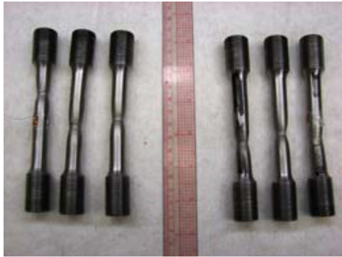
Figure 67. Necking behavior observed in the TC128B round bar specimens.
