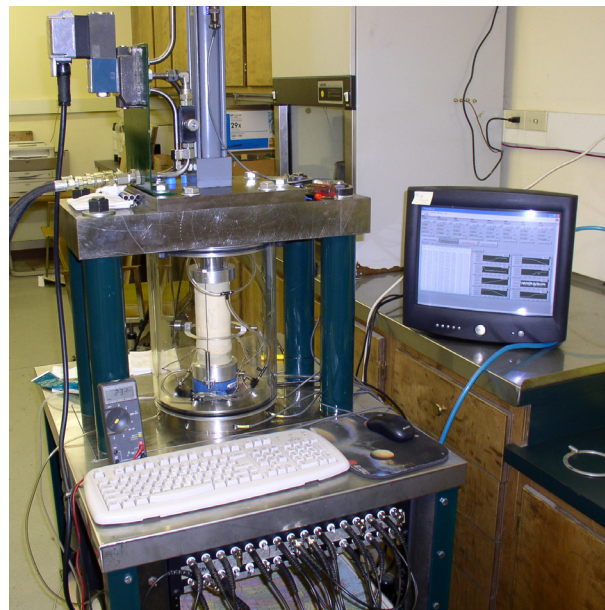
Figure 206. Schematic and photograph of the triaxial compression test apparatus.
