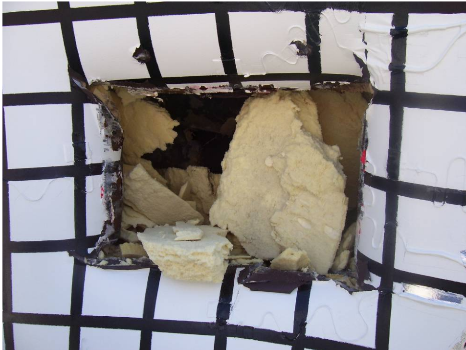
Figure 244. Puncture of the external protective layers in Head Test 2.
