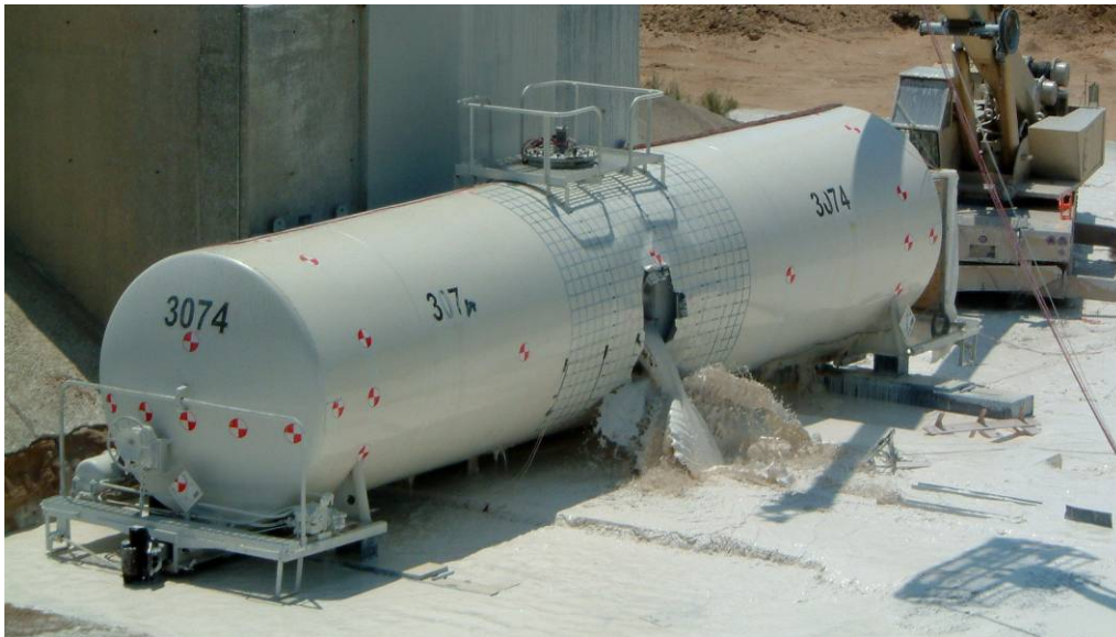
(b) Post-test tank damage
