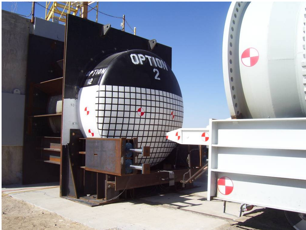
Figure 243. Pretest configuration of the test head and ram car.
