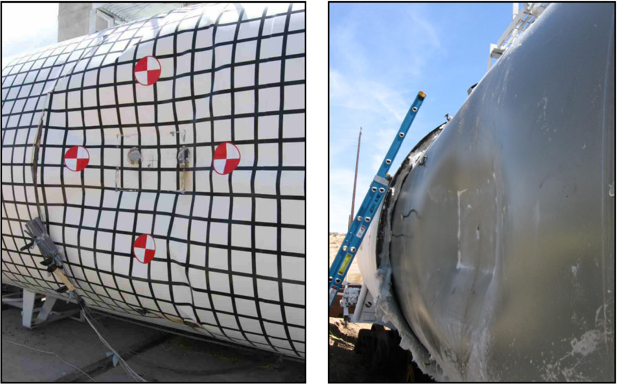
Figure 37. Post-test dents in the jacket and shell of Tank Car 3069
