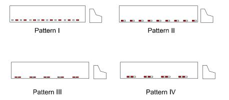
**Truck** Figure 2. Truck Retroreflective Patterns
