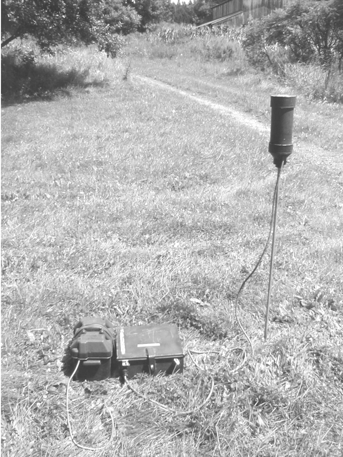
Figure 7. Photograph Showing the Long-Term Measurement Configuration. The EMF Sensors are Situated in the Cylindrical PVC Unit and Connected to the MultiWave System II Data Acquisition Equipment in the Weatherproof Container. Power is Supplied from a 12-Volt Battery at the Left
