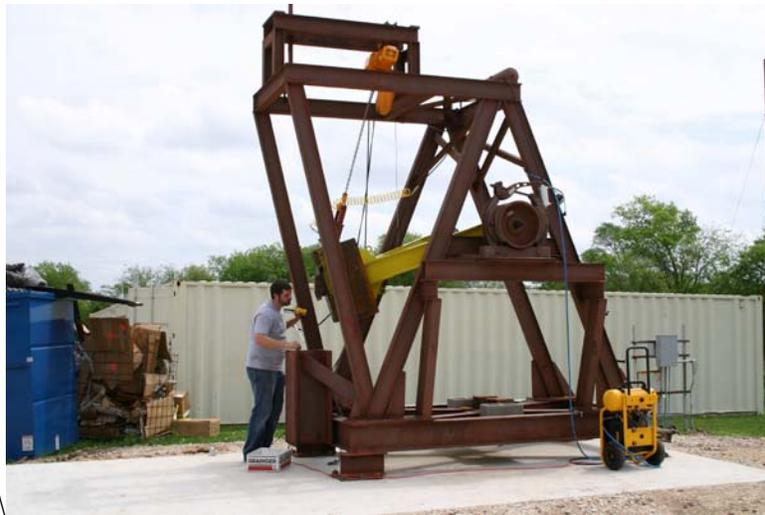
**Figure 66. Oversized, Nonstandard Pendulum Impactor**
