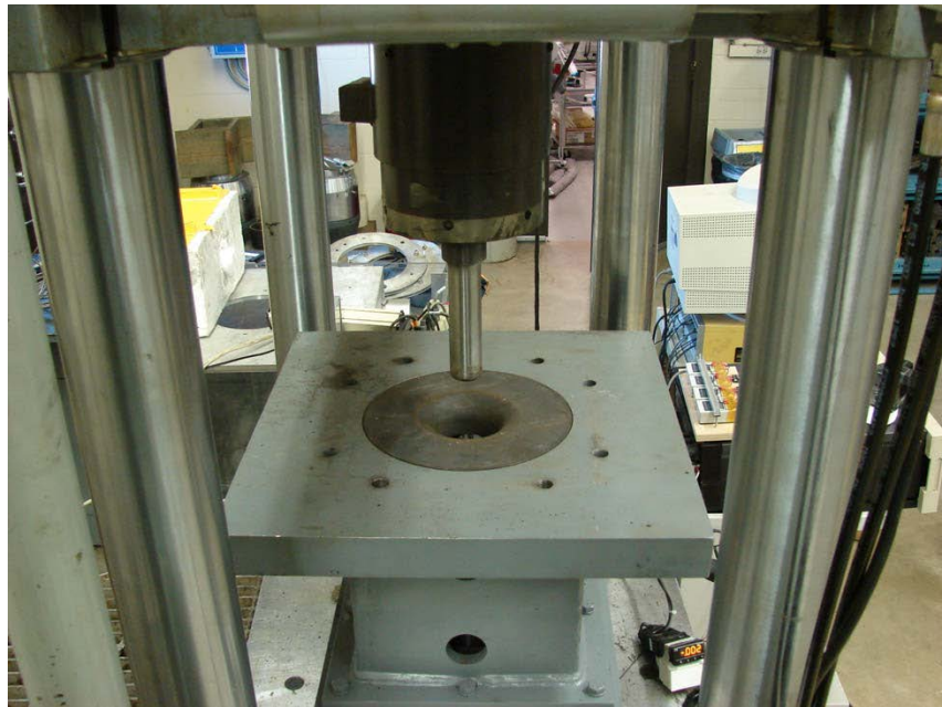
Figure 39. Simulation of the Punch Test on the Thin TC128B Plate Material
