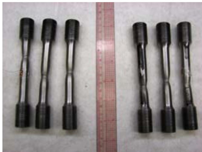
Figure 31. Necking Behavior Observed in the TC128B Round Bar Specimens
