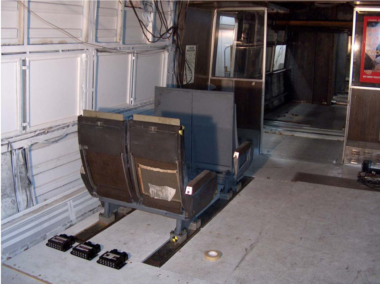
Figure 30. Plywood Floor Installed around Experiment 2.1
