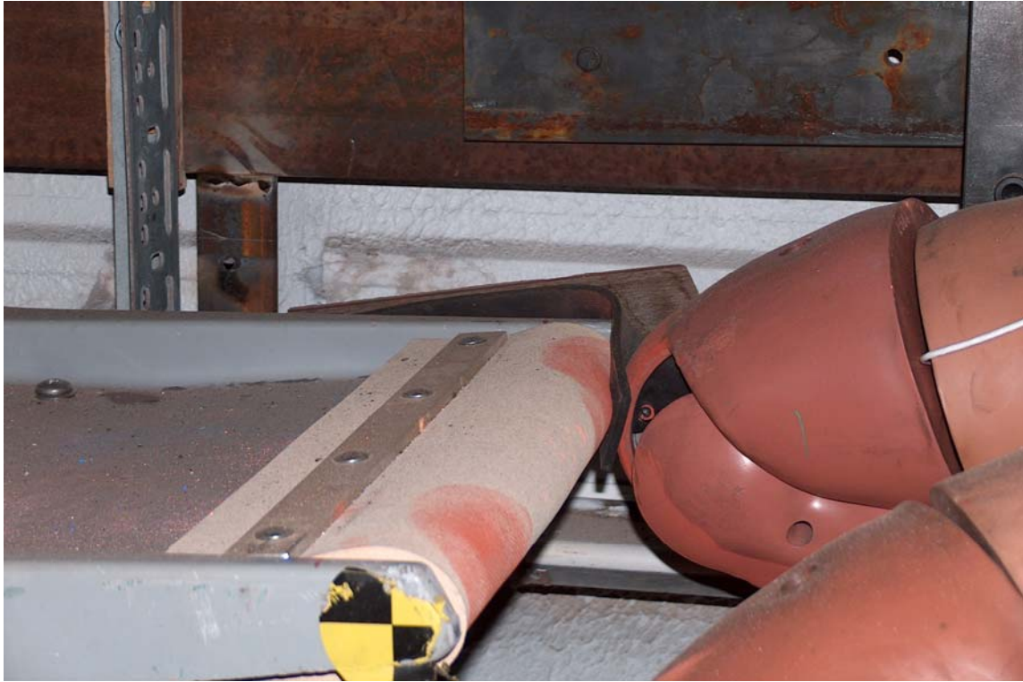
Figure 49. Interaction of the Knees with the Facing Seat Rubber Bumper Occured in Experiment 1.2
