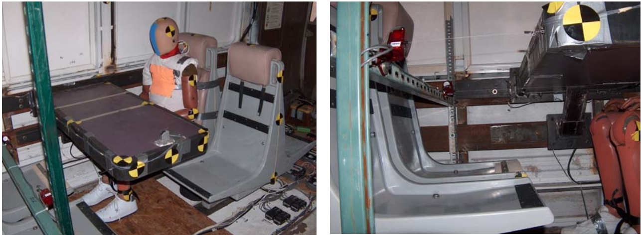
Figure 20. Table Acceleration was Measured with an Accelerometer, and Table Crush and Displacement were Measured with Two Potentiometers
