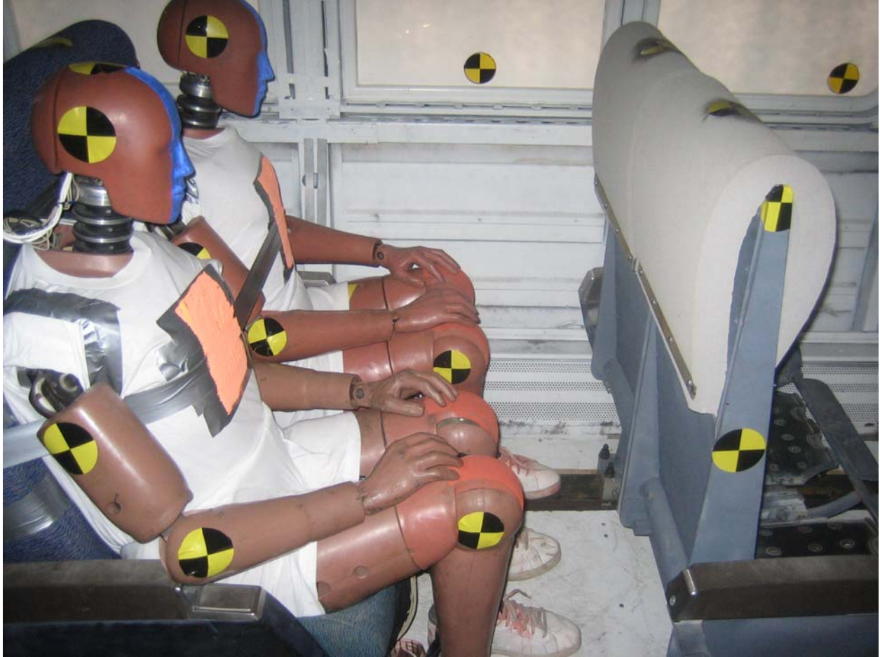
Figure 33. Two Instrumented Hybrid III 95th Percentile ATDs Occupied the Two-Place Passenger Intercity Seat in Experiment 2.1
