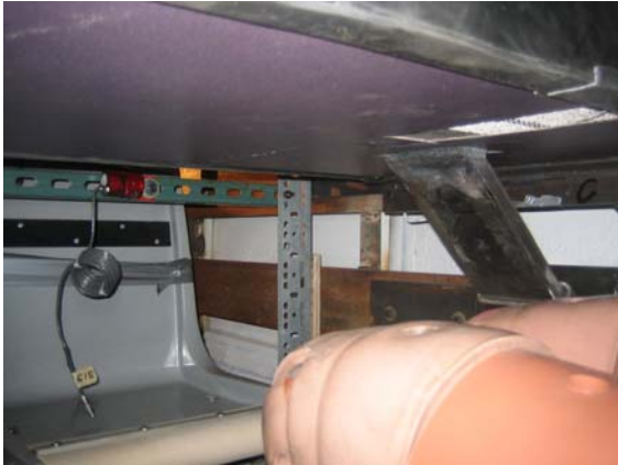
Figure 21. Potentiometer Cord for Table Crush, Stretched under Table to a Hook Bonded into the Honeycomb Where a Melamine Strip was Removed (left). Cord for Table Displacement, Stretched from the Unistrut to a Hook Bonded into the Facing Edge of the Table (right) in Experiments 1.2 and 1.3
