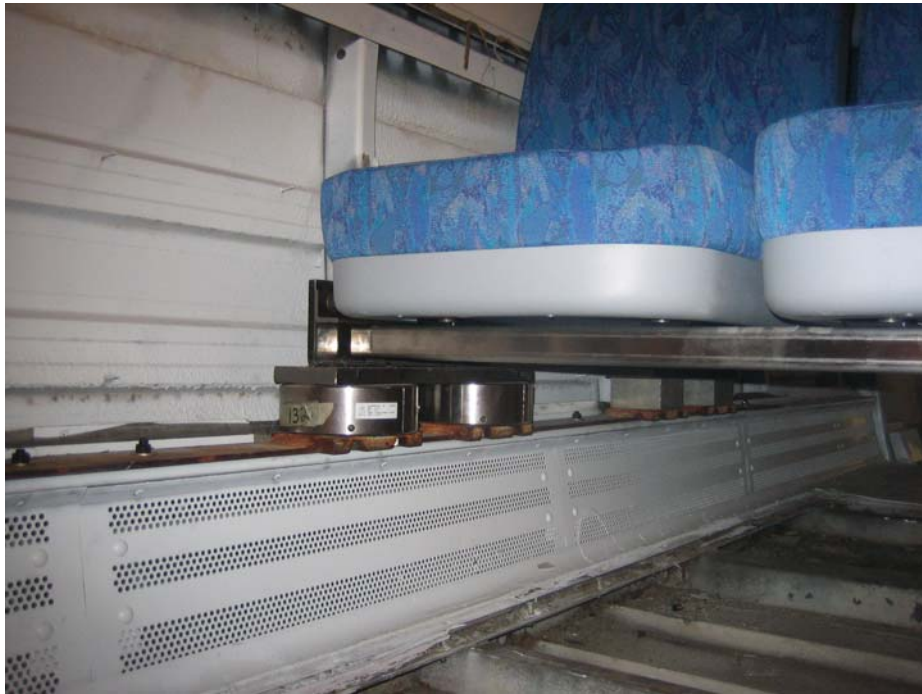
Figure 38. Rugged Angle Iron was Bolted to the Vertical Piece of the T-Shaped Load-Cell Attachment Plate, Then Bolted to the C-Channel That Formed the Base of the Seat Assembly
