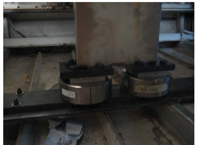
Figure 5. Floor-Attachment Spacer Blocks for Unoccupied Rebound Seat (left) and Load Cells for Occupied Front-Row Seat (right) in Experiment 1.1
