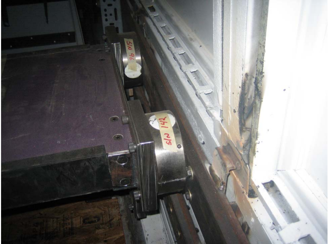
Figure 18. Table Bolted to Three Individual Attachment Plates which were Bolted to the Load Cells
