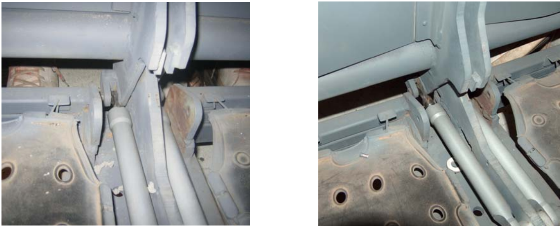
Figure 54. Energy-Absorbing Struts Before the Test (left), Actuated Approximately 0.75 in (right) to Help Reduce the Force of the Head Impacting the Seat Back
