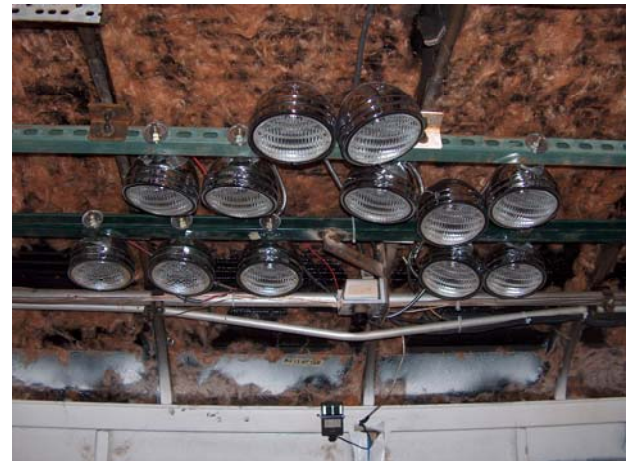
Figure 23. Twelve Flood Lights and One U512 Camera, were Installed above for Experiment 1.2 (left) and Experiment 1.3 (right)
