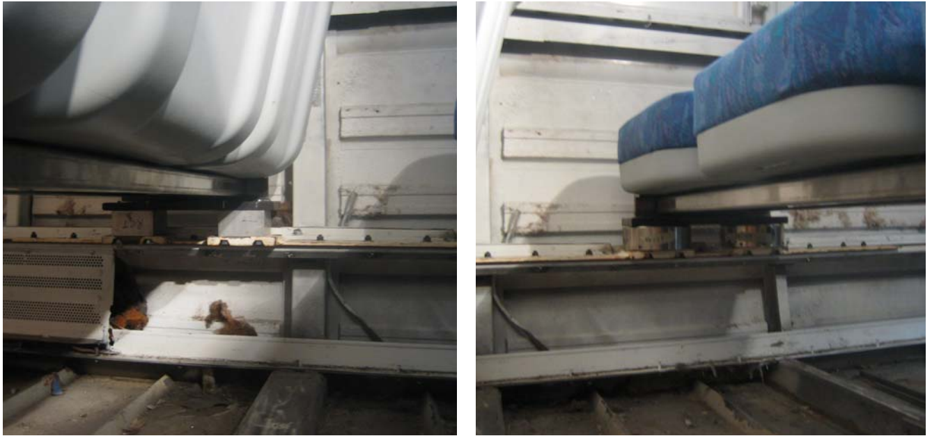
Figure 6. Wall-Attachment Spacer Blocks for Unoccupied Seat (left) and Load Cells for Occupied Seat (right) in Experiment 1.1
