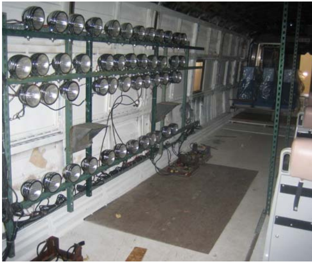
Figure 22. Forty-Eight Flood Lights were Installed along the Wall (left), with Two RS Cameras (right) Covering Both Experiments 1.2 and 1.3
