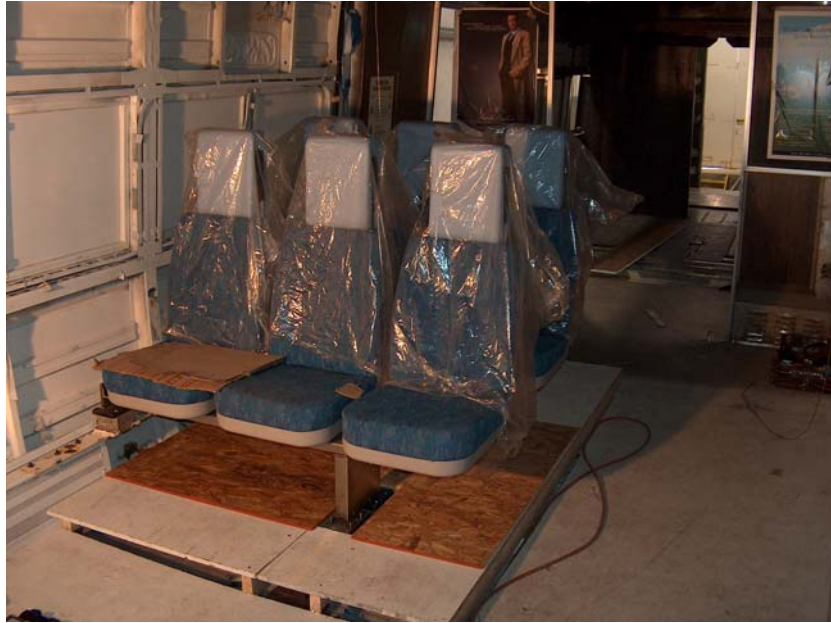
Figure 39. Plywood Floor Built around the Seat Installation Raising the Floor to the Level Where the Pedestal Base was Installed in Experiment 2.2
