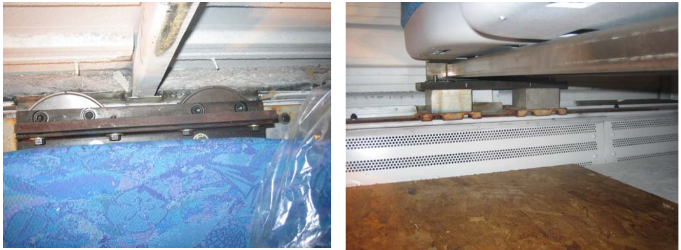
Figure 37. Top View of the Wall-Attachment Load Cells on the Unoccupied Impact Seat (left), and Underside View of Spacer Blocks on the Launch Seat (right) in Experiment 2.2
