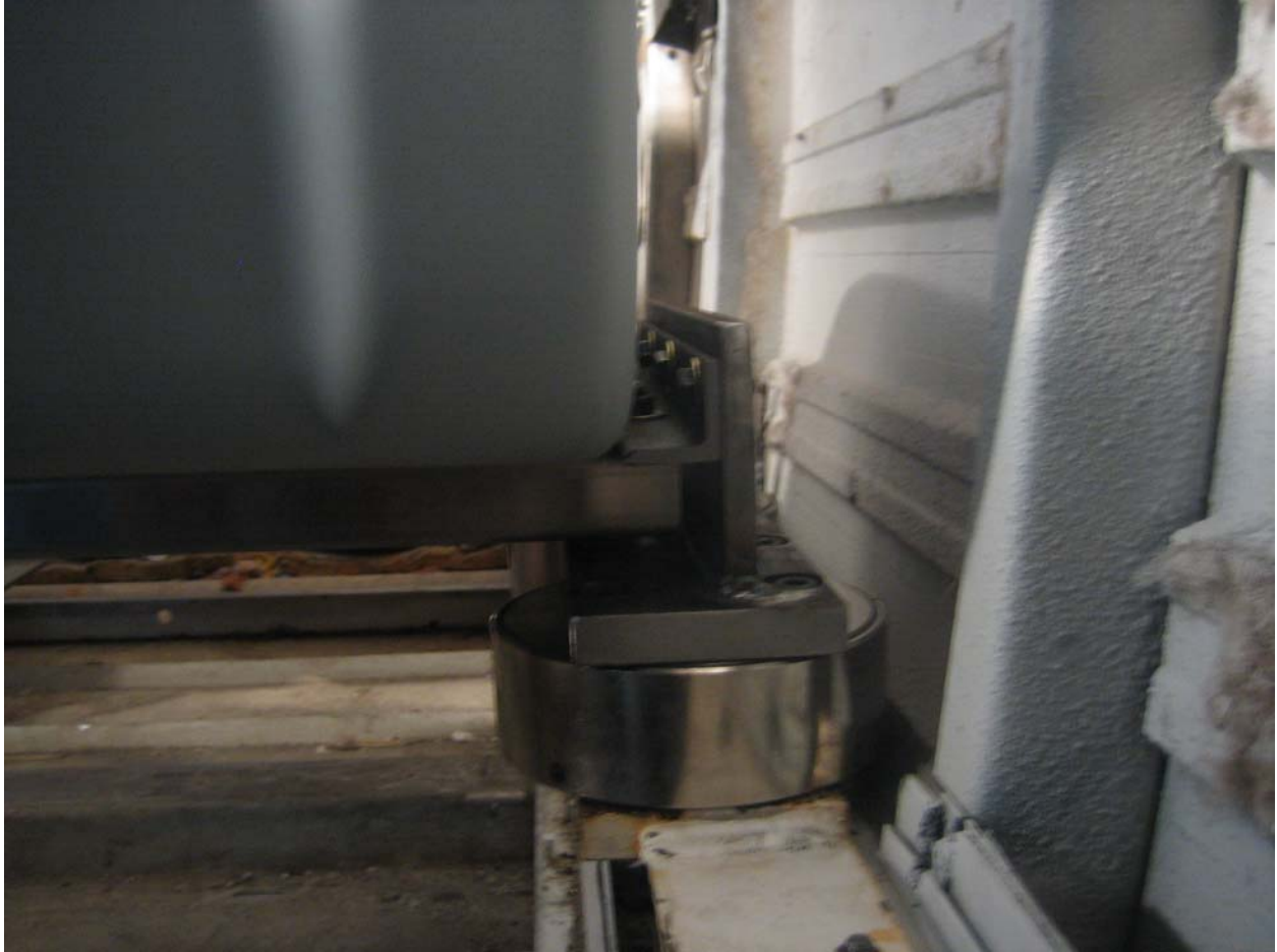
Figure 7. Rugged Angle Iron Bolted to the Vertical Piece of the T-Shaped Load-Cell Attachment Plate and Bolted to the C-Channel That Formed the Base of the Seat Assembly
