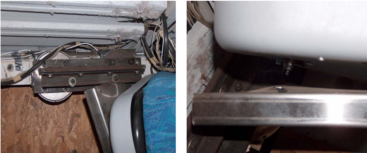
Figure 47. The Bolt Holding Seat Base at the C-Channel Pulled through. The Connection Holding the C-Channel to the Wall also Failed
