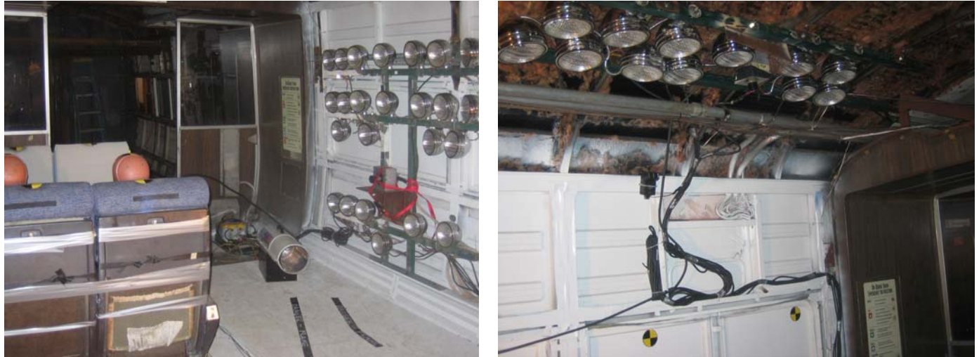
Figure 32. One APX Camera and 24 Flood Lights were Installed along the Wall (left) and One U512 Camera and 12 Lights were Installed along the Ceiling (right) in Experiment 2.1
