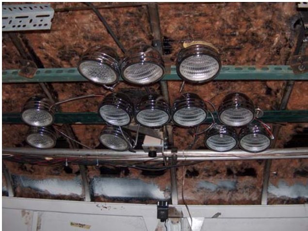
Figure 23. Twelve Flood Lights and One U512 Camera, were Installed above for Experiment 1.2 (left) and Experiment 1.3 (right)
