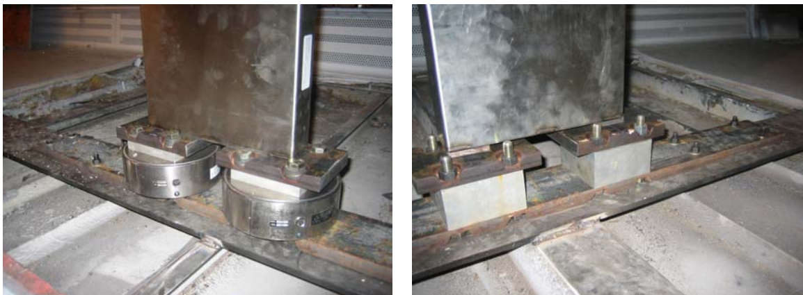
Figure 36. Floor Attachment Load Cells for the Impact Seat (left) and Spacer Blocks for the Launch Seat (right) in Experiment 2.2
