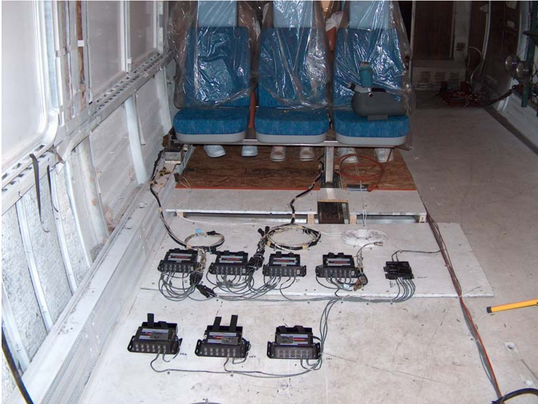
Figure 9. Four Data Bricks Installed behind the Aft-Facing Seating Experiment to Collect 29 Channels of Data in Experiment 1.1
