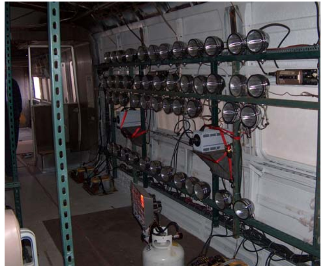
Figure 22. Forty-Eight Flood Lights were Installed along the Wall (left), with Two RS Cameras (right) Covering Both Experiments 1.2 and 1.3
