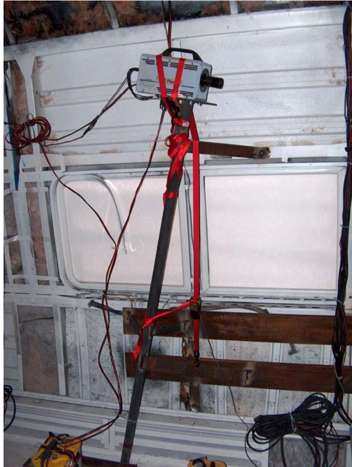
Figure 24. One RS Front View Camera was Installed to Capture the Combined Front View of Experiments 1.2 and 1.3
