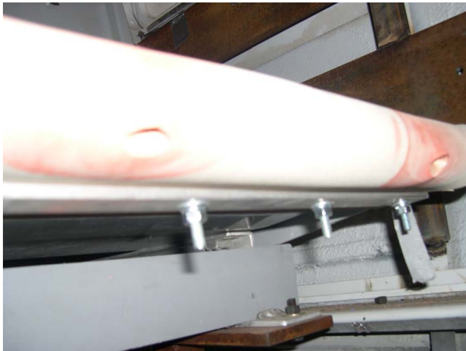
Figure 52. Tears in the Rubber Bumper from Knee Interaction with the Facing Seat in Experiment 1.3
