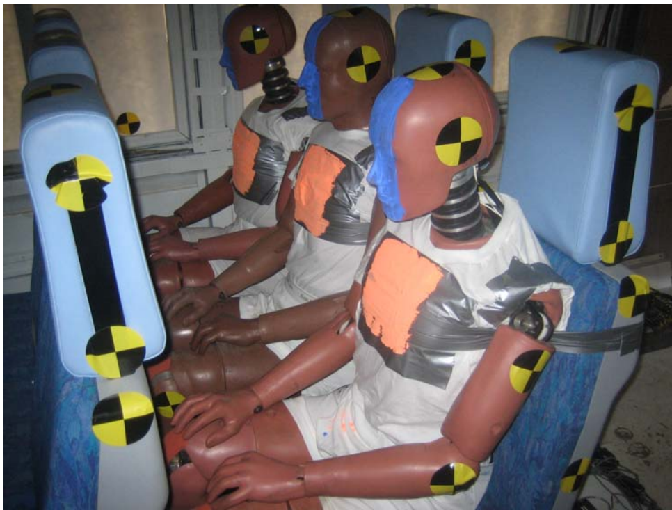
Figure 42. Instrumented Hybrid III ATDs Occupied the Aisle and Window Seats. An Uninstrumented Hybrid II ATD Occupied the Middle Seat in Experiment 2.2
