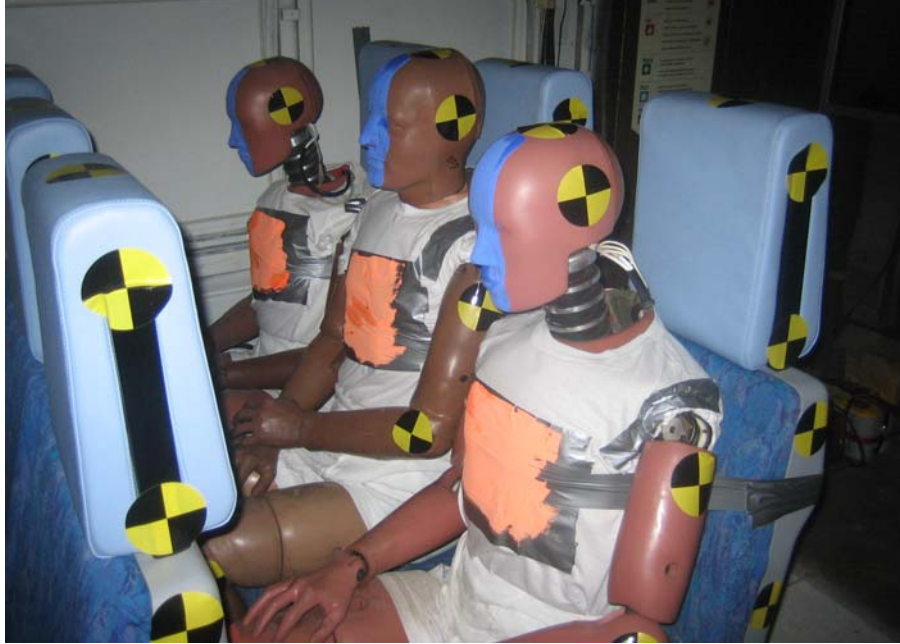
Figure 11. Reference Targets Placed on Each ATD at the Head, Shoulder, Elbow, and Knee Locations, and on the Seats along the Edge of the Headrest and Seat Back
