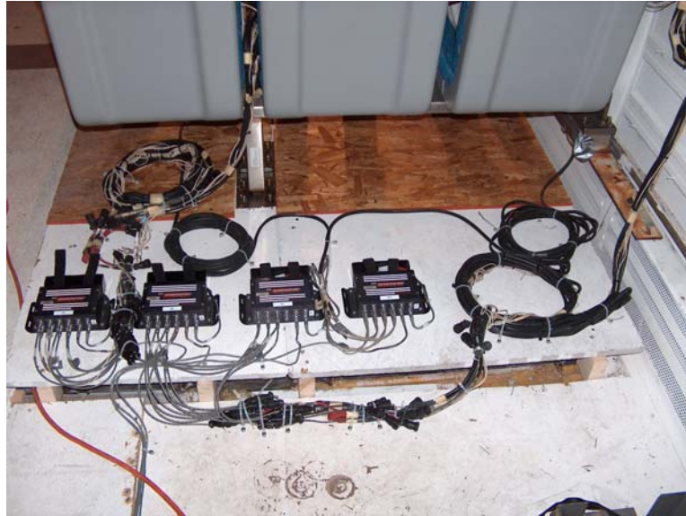
Figure 40. Four Data Bricks Installed Behind Experiment 2.2 to Collect 32 Channels of Data
