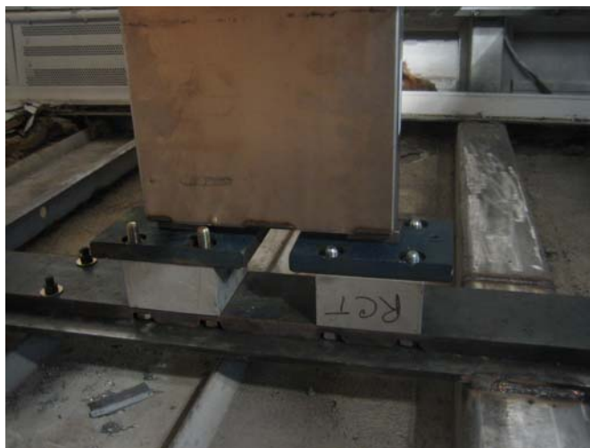
Figure 5. Floor-Attachment Spacer Blocks for Unoccupied Rebound Seat (left) and Load Cells for Occupied Front-Row Seat (right) in Experiment 1.1
