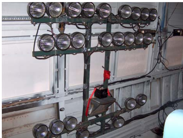
Figure 41. One U512 Camera and 24 Flood Lights Were Installed along the Wall and One U512 Camera and 12 Lights Were Installed along the Ceiling
