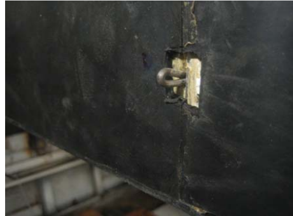
Figure 21. Potentiometer Cord for Table Crush, Stretched under Table to a Hook Bonded into the Honeycomb Where a Melamine Strip was Removed (left). Cord for Table Displacement, Stretched from the Unistrut to a Hook Bonded into the Facing Edge of the Table (right) in Experiments 1.2 and 1.3
