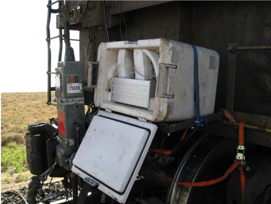
**Figure H-7. Rear Car Instrumentation Data Acquisition Computer**
