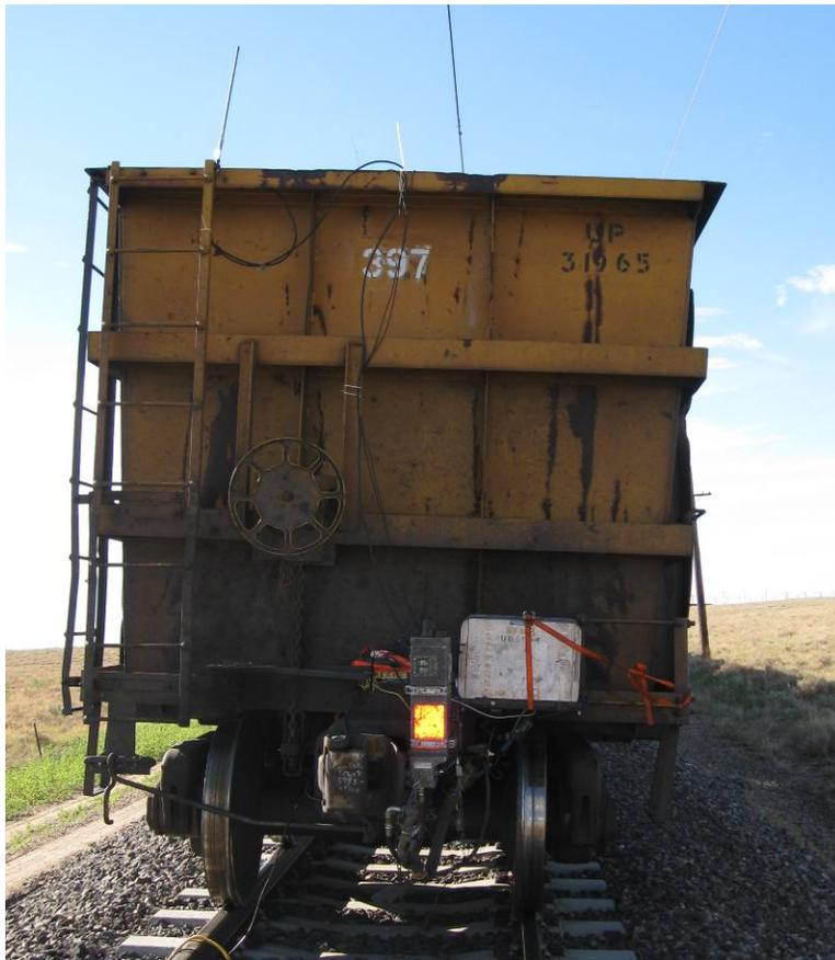
**Figure H-6. Rear Car Instrumentation including EOT, Data Acquisition Computer, and Antenna**
