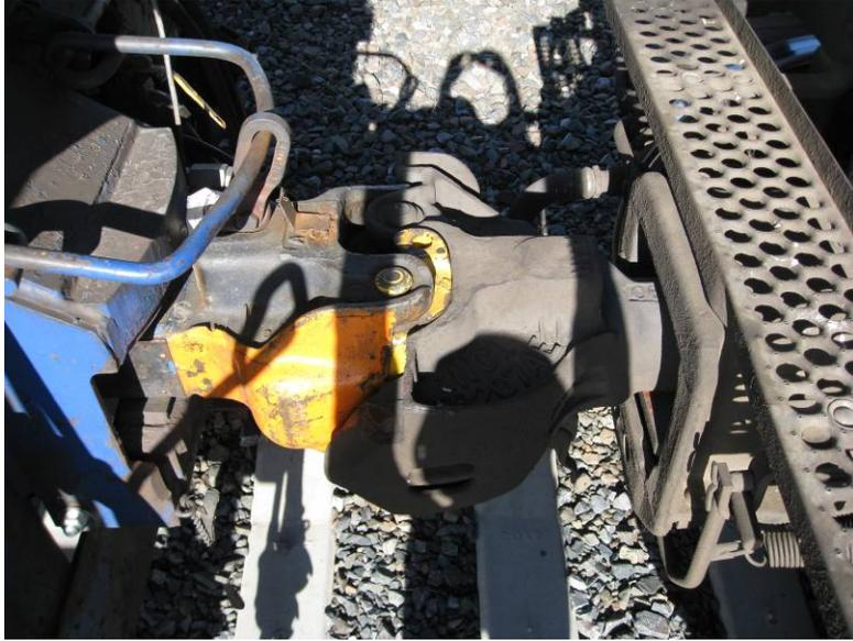
**Figure H-5. Instrumented Coupler Installed on Rear Locomotive**
