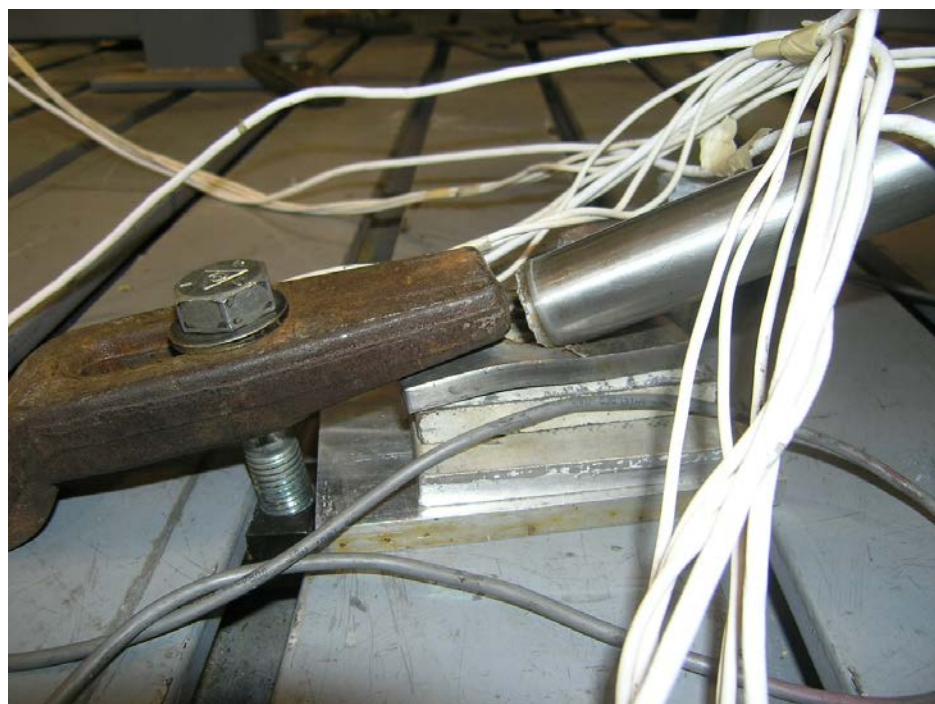
Figure 20. Post-Test Photograph of Sheared-Away Floor Pedestal
