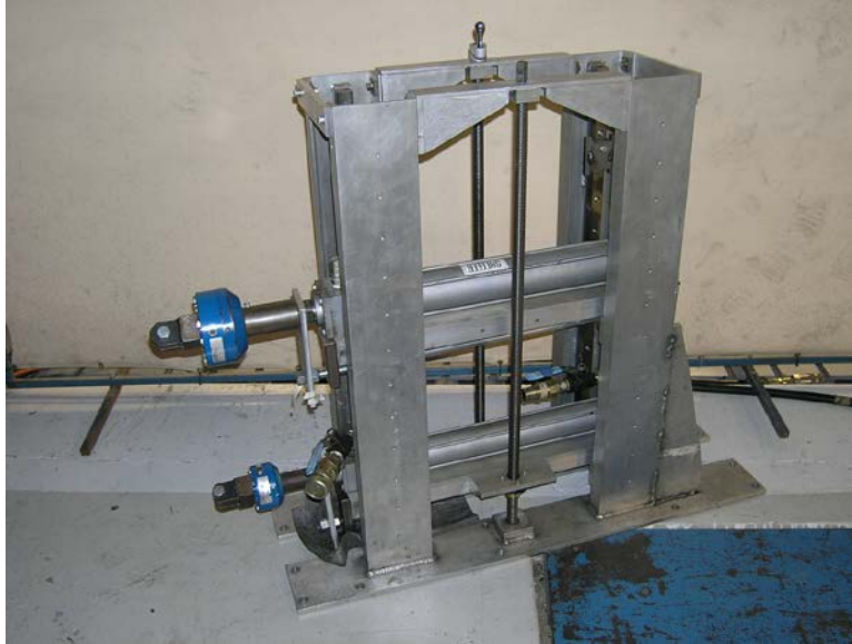
Figure A1. Example Structural Loading Frame
