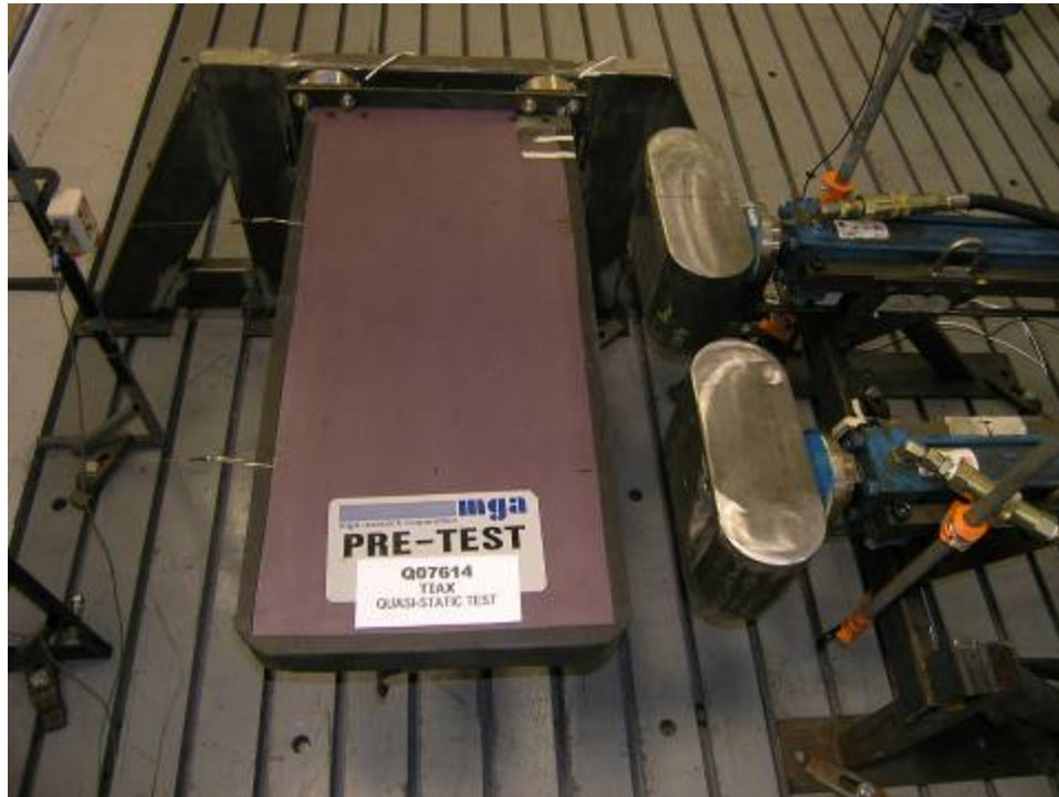
Figure 4. The Instrumented Workstation Table Prior to the Quasi-Static Test
