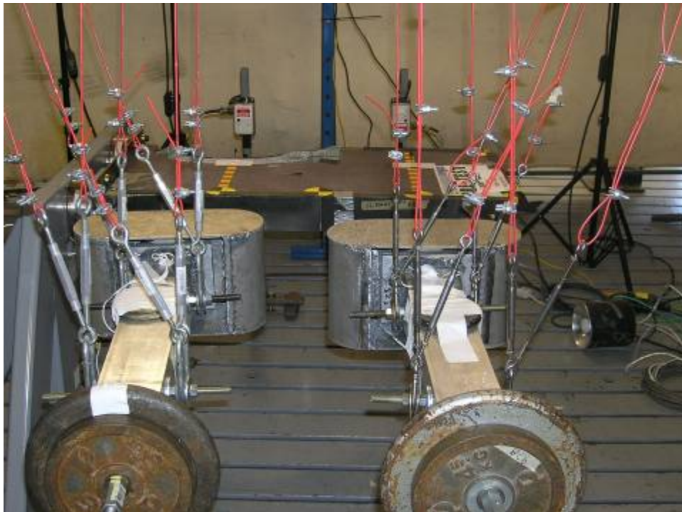
Figure 9. Arrangement of Pendulum Cables
