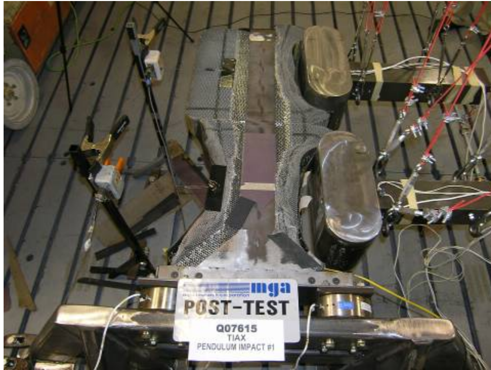
Figure 11. Side View of the Instrumented Workstation Table Following the First Dynamic Pendulum Test
