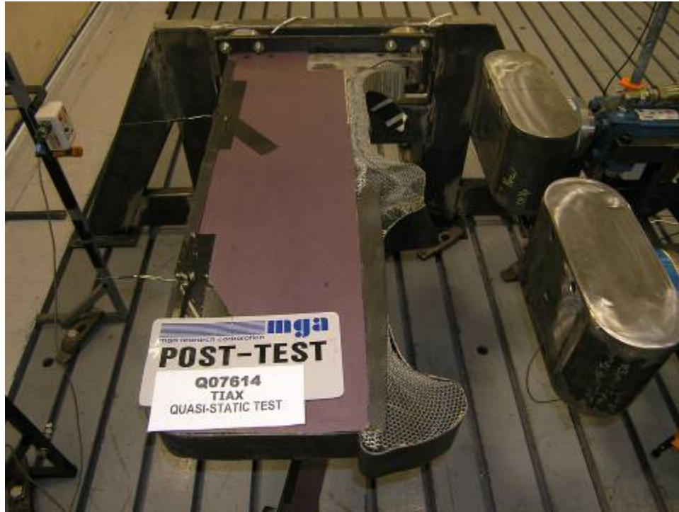
Figure 6. The Instrumented Workstation Table Following the Quasi-Static Test
