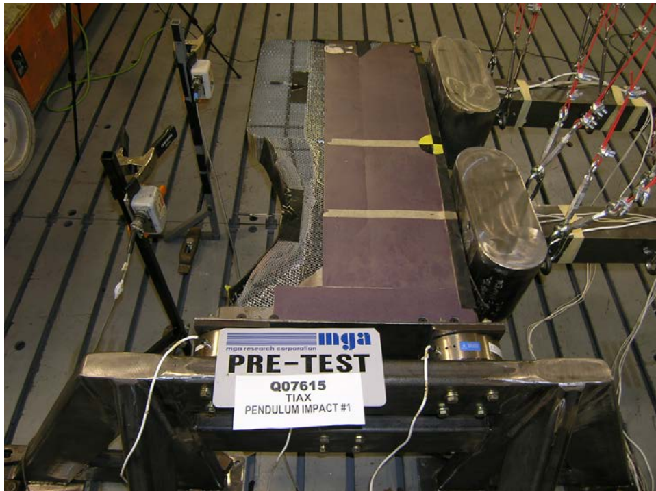
Figure 10. Side View of the Instrumented Workstation Table Prior to the First Dynamic Pendulum Test
