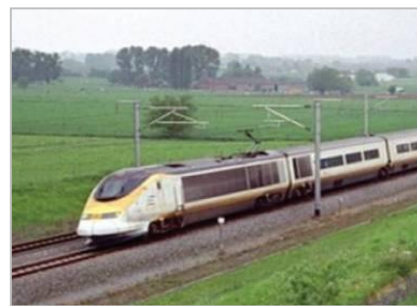
Figure 2-3 Example of an at-grade profile showing contact wire system and vertical arms of the pantograph power pickups
