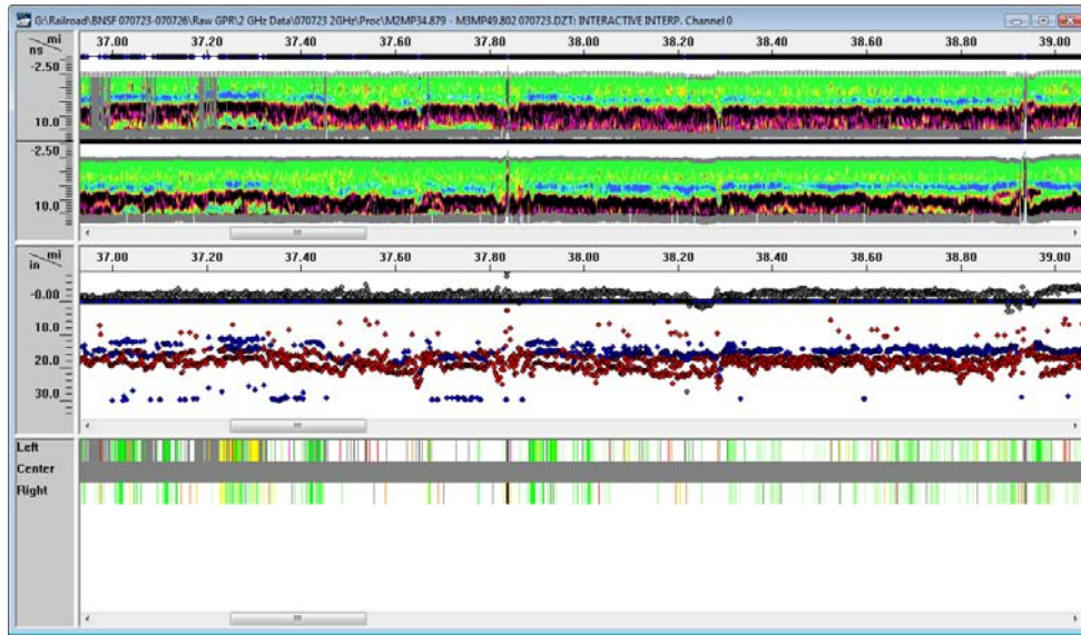
Figure 59. Processed 2 GHz data obtained between MP37 and 39 on track Main 2 before a rainfall event.
