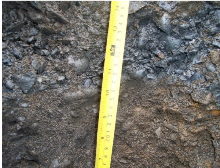
Figure 70. Layer of distinct blue-gray crushed stone that is typically near 24-inches deep at most ground truth locations. The moisture content of the subballast beneath this layer was substantially higher.
