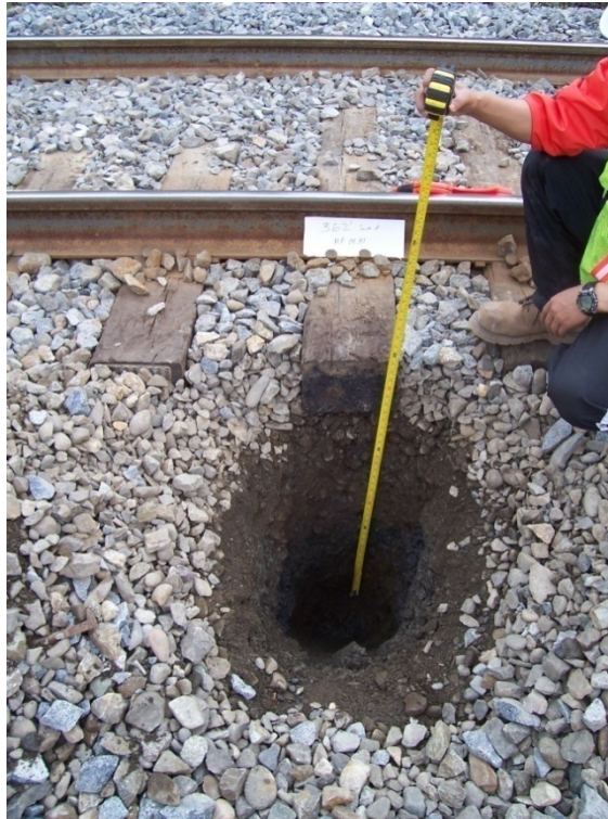
Figure 69. Typical ground truth hole. The depth of this hole relative to the top of the tie was 3 ft.
