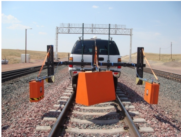
Figure 50. Data collection setup. Two 2 GHz horn antennas were mounted on the shoulders and a 500 MHz horn antenna was mounted between the rails.
