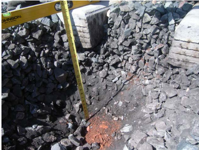
Figure 51. Typical ground truth hole. Pink material at bottom is top of the subballast.
