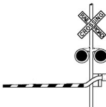
**Figure B-5. An automatic gate device with flashing lights.**
