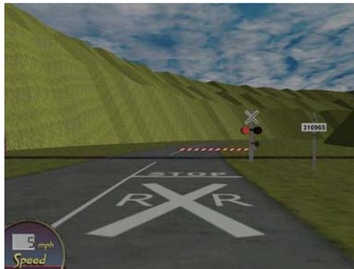
**Figure B-1.** An example of an active grade crossing.
