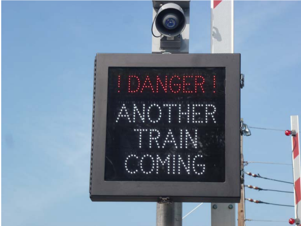
Figure 1. Another Train Coming Warning Sign and Auditory Alert Speaker
