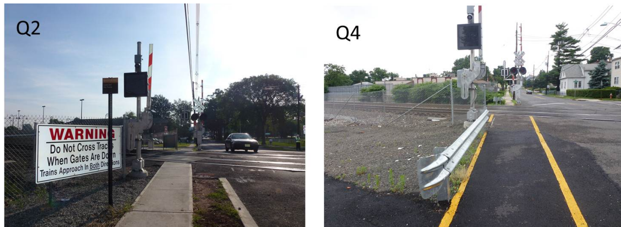
Figure 10. Another Train Coming Signage Placement in Q2 and Q4
