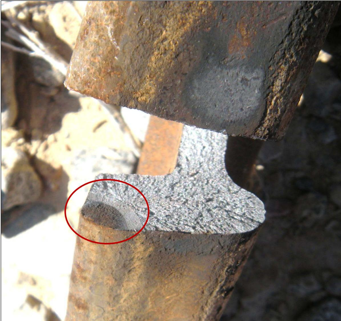
**Figure 18. Typical Fatigue Crack in the Bottom of the Joint Bar**
