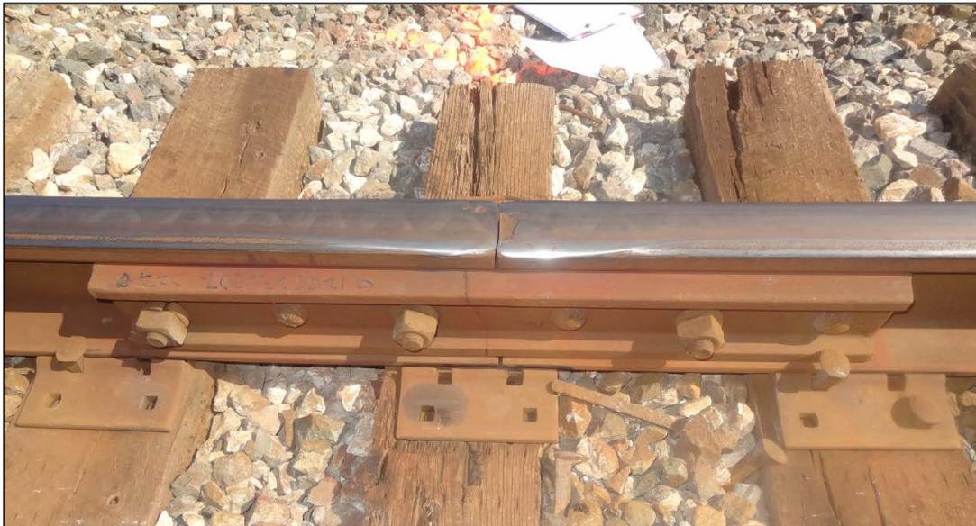
**Figure 1. A Broken Joint Bar in Service**
