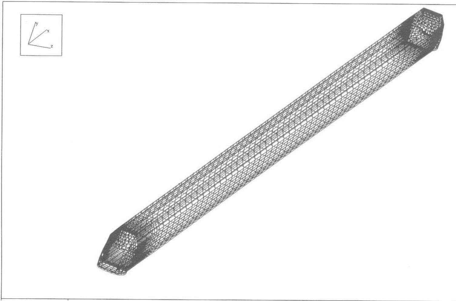
Figure 3-4. CFD Model – Acela Trainset Computational Grid – Grid (157 x 31 x 41)
