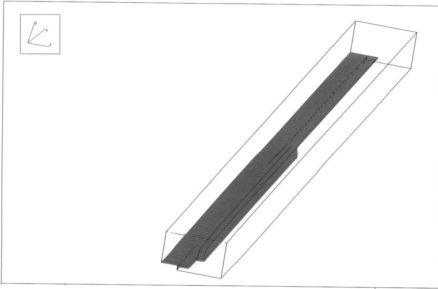
Figure 3-2. CFD Model – Isometric View – Acela Trainset Next to Platform – Grid (157 x 31 x 41) – Dimension (1322 x 40 x 67) ft
