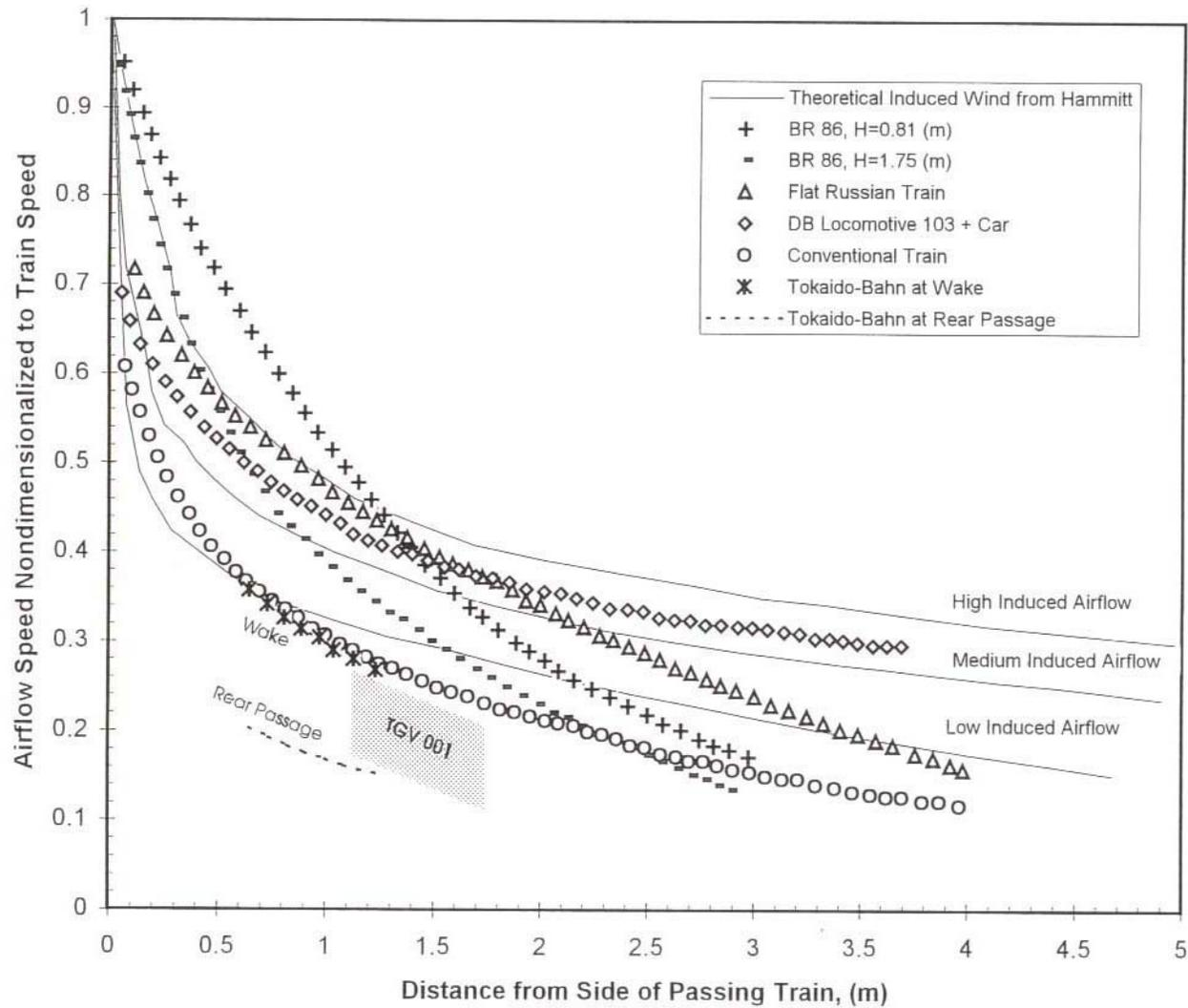
Figure 2-1. Theoretical and Experimental Induced Airflow Speed From a Passing Train, From Lee (1999)
