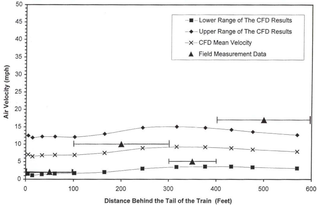
Figure 4-1. Comparison of CFD Analysis with Measured Airflow Velocities at Princeton Junction, NJ, at 9 ft from Side of Train – 5 ft Above Equivalent Low-Level Platform Condition (Rail/Ground) – CFD Train Speed = 125 mph, Field Train Speed = 125 +/- mph.
