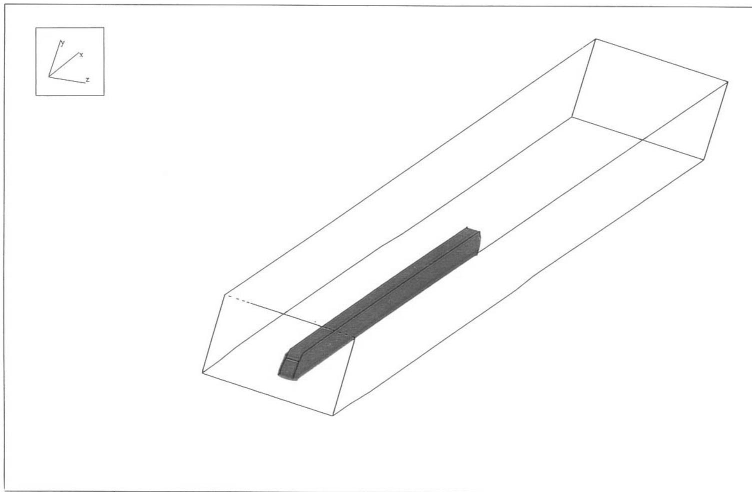
Figure 3-1. CFD Model – Isometric View – Acela Trainset with Low-Level Platform (at ground level) – Grid (157 x 131 x 41) – Dimension (1322 x 40 x 67) ft
