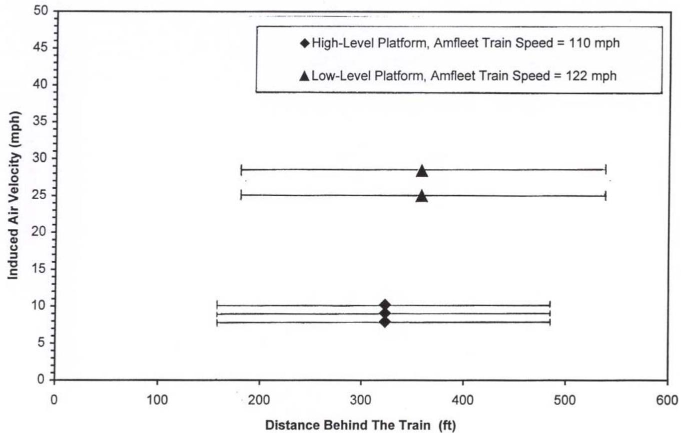
Figure 4-3. Comparison of Measured Air Velocities for Low versus High-Level Platform at 9 ft from Side of Train – 5.5 ft Above Platform Level – Low-Level Platform at Newark, DE and High-Level Platform at Princeton, Junction, NJ
