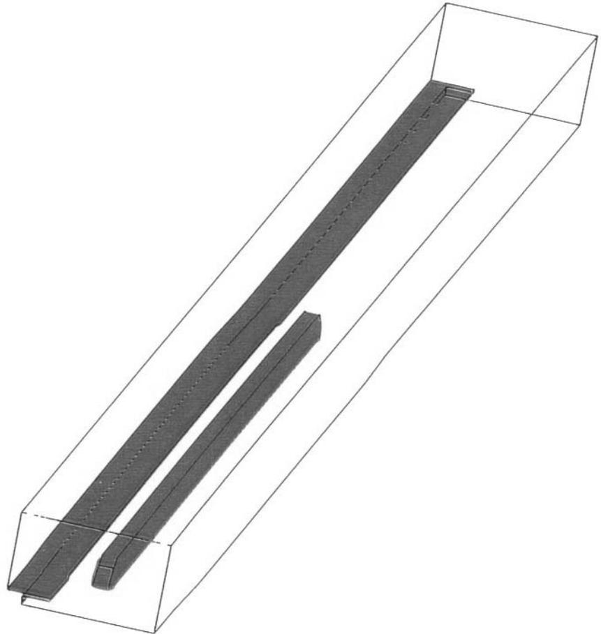
Figure 3-3. CFD Model – Isometric View – Acela Trainset Second Track From Platform – Grid (157 x 31 x 41) – Dimension (1322 x 40 x 67) ft
