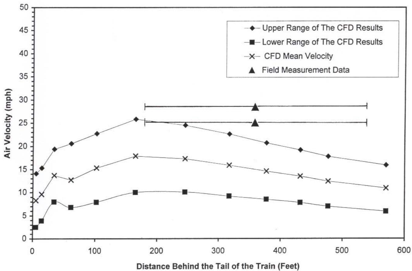
Figure 4-2. Comparison of CFD Analysis with Measured Airflow Velocities at Newark, DE – 5.5 ft from Side of Train – 5.5 ft Above Low-Level Platform – CFD Train Speed = 125 mph, Field Train Speed = 122 +/- mph
