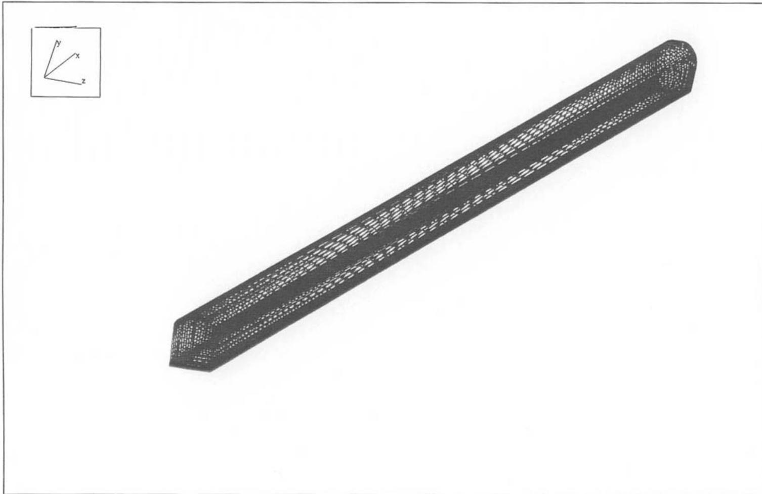
Figure 3-20. CFD Model – Amfleet Trainset Computational Grid - Grid (160 x 38 x 53)
