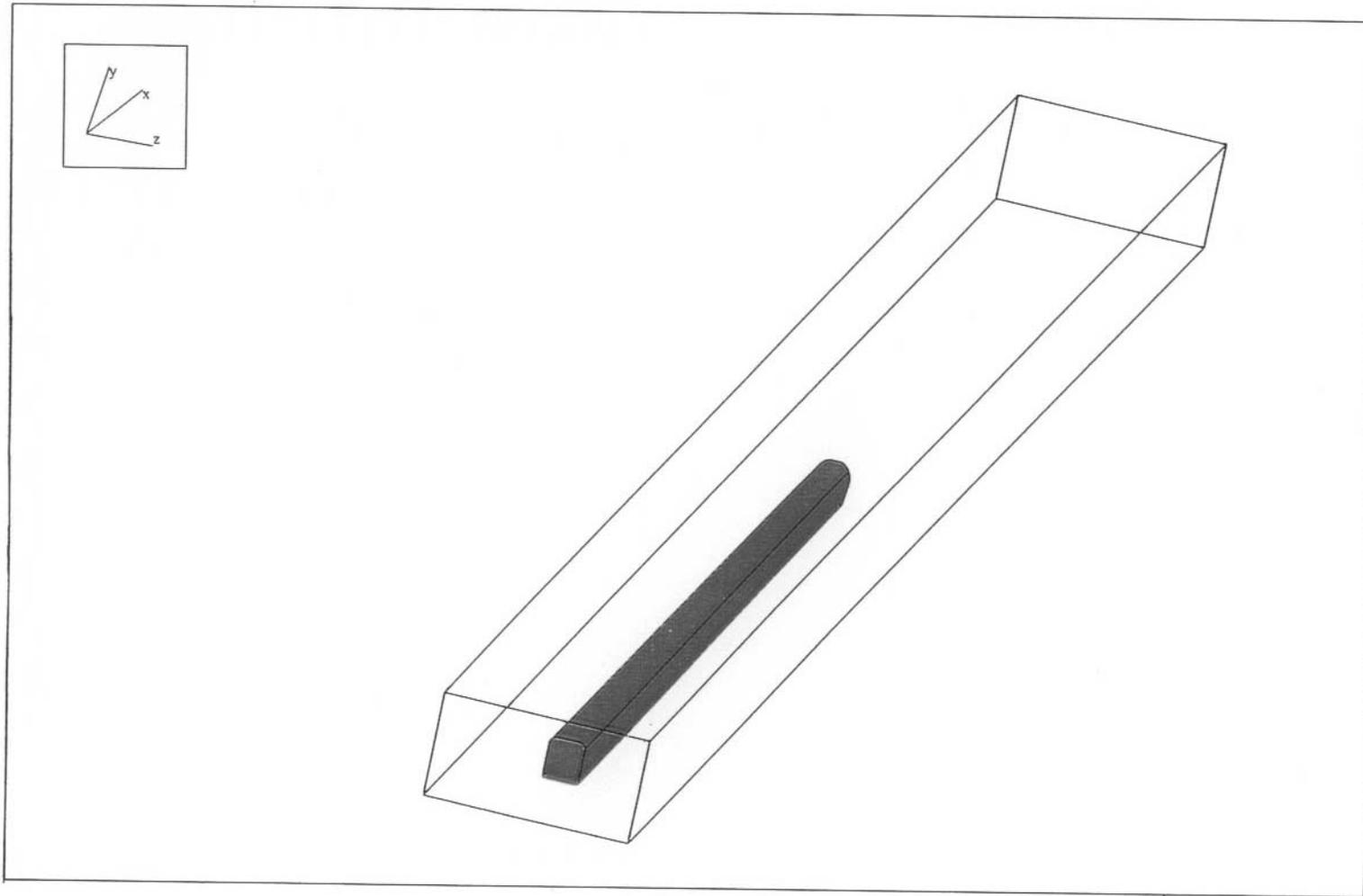
Figure 3-19. CFD Model Isometric View – Amfleet Trainset with Low-Level Platform – Grid (160 x 38 x 53) – Dimension (1200 x 40 x 60) ft
