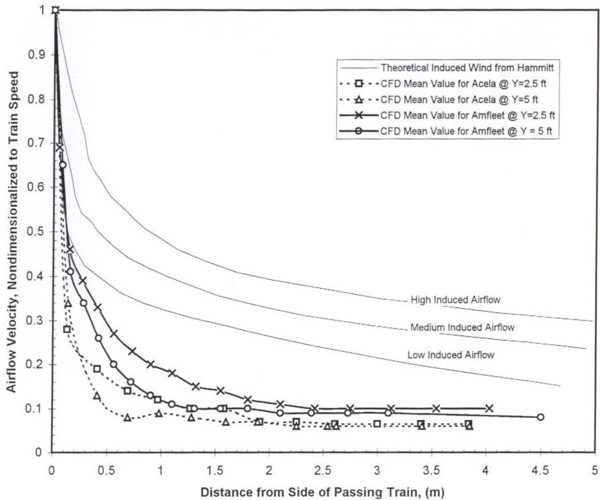
Figure 3-24. Results from CFD Model versus Theoretical Results from Hammitt (1973) for Induced Airflow Velocity from a Passing Train, Excerpted from Lee (1999)
