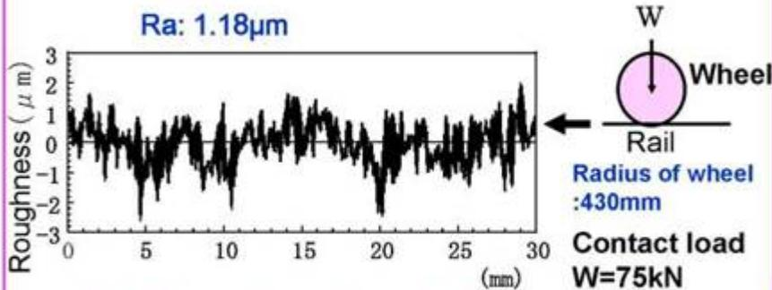
Configuration of equivalent roughness between wheel and Rail
