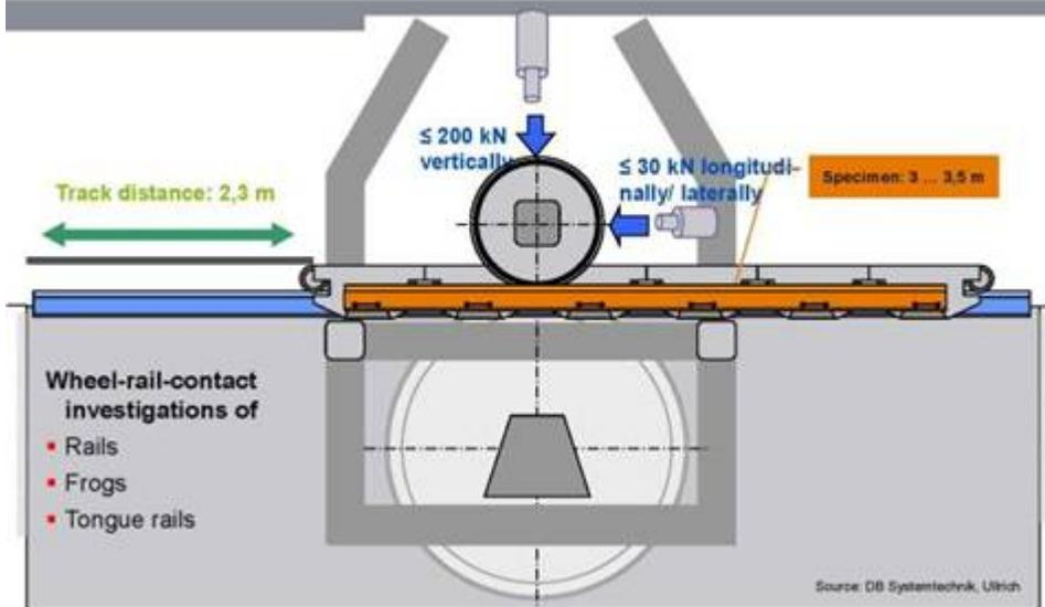
**Material testing on the wheel-rail-system test stand**
