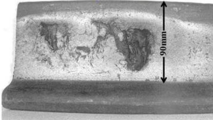
Crack is caused by formation of white etching layer and water
