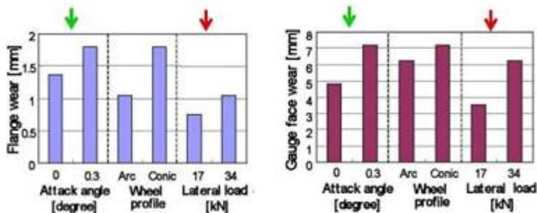
(a) Flange wear amount at  $1.68 \times 10^6$  cycles corresponding to 2638km of running distance
