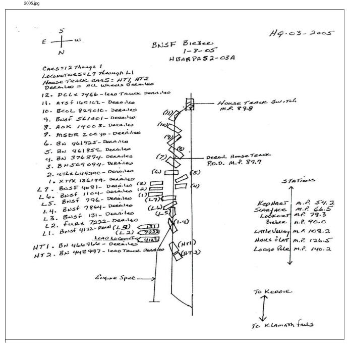
108. DRAW A SKETCH OF ACCIDENT AREA INCLUDING ALL TRACKS, SIGNALS, SWITCHES, STRUCTURES, OBJECTS, ETC., INVOLVED. HQ-03-
