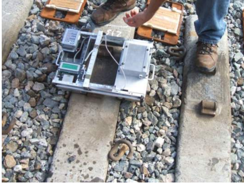
Figure 5. Automated RSA Profile Data Collection System Prototype Used to Collect the Perimeter Depth and Pattern of RSA
