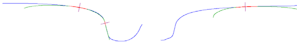
Figure 35. Wheel/Rail Contact Geometry for Axle 2 at 345 ft along the Track for MP 584.5, with Corresponding Left and Right Wheel L/V Ratios
