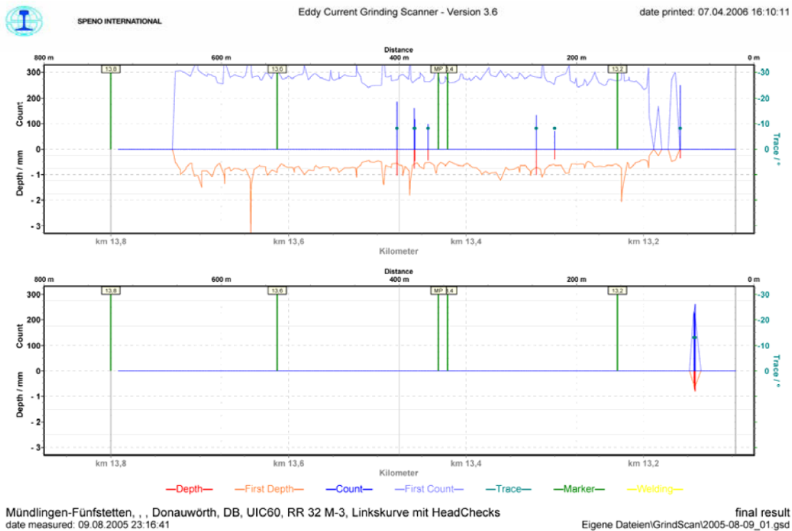
Figure 38. Example Plot of Processed Data from the Speno Rail HC Grinding Scanner System
