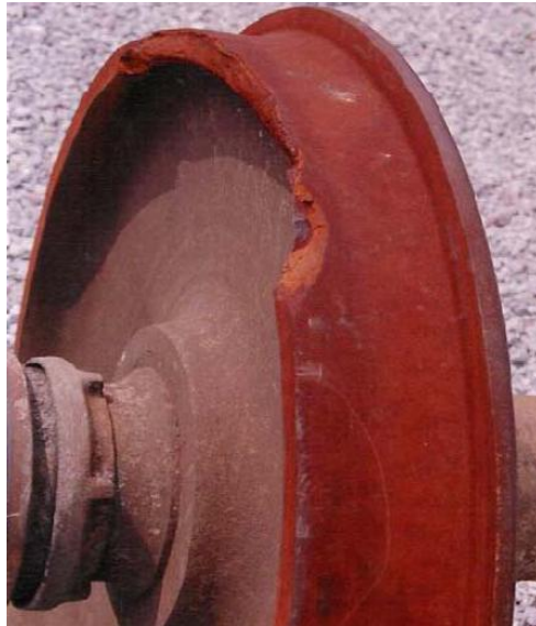
Figure 17. A Typical Vertical Split Rim [260]
