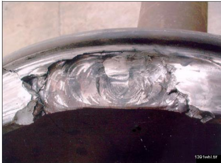
Figure 16. A Shattered Rim Failure [262]
