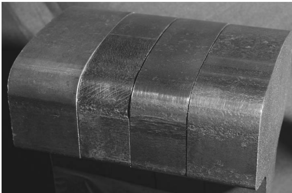
Figure 56. The Effect of Friction Management of Wear and RCF – Full-Scale Rig Test Results; Left to Right: New 60E1 Profile, “Dry” after 100k Wheel Passes, FM 100k Wheel Passes, and FM 400k Wheel Passes (from Reference 257)
