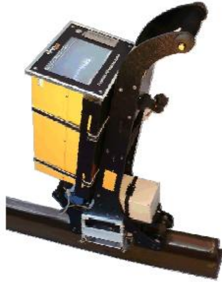
B) NEWT Eddy Current based walking stick
