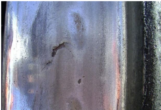
E) Incipient shells initiating at the field/rim side of the wheel.
